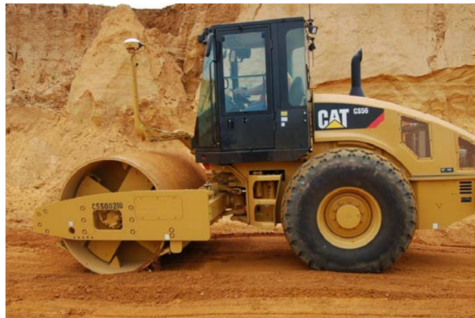
Figure 3.6 Caterpillar CS56 vibratory smooth drum roller (Tehrani 2009).
