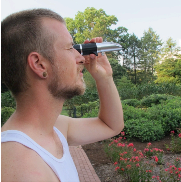
Figure 3.5 The author observing sugar concentration using a handheld refractometer. Photo courtesy of Jennifer James
