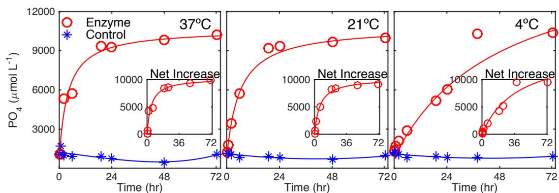
Figure 6 Phosphate released from poly-P degradation by acidic phosphatase enzyme from wheat. Poly-P was incubated under three different temperatures (37 °C, 21 °C, and 4 °C).
