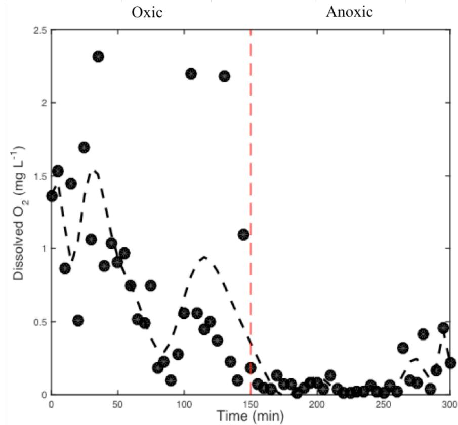
Figure 12 Dissolved oxygen concentration in KCRWTF aeration basin within 300 min (one oxic-anoxic cycle). The pumping of air was stopped at ~150 min (data from March 2016).
