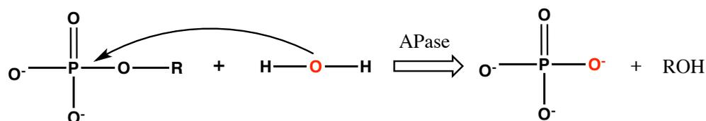
Figure 4 Mechanism of phosphomonoester hydrolysis catalyzed by alkaline phosphatase (Liang and Blake, 2009).
