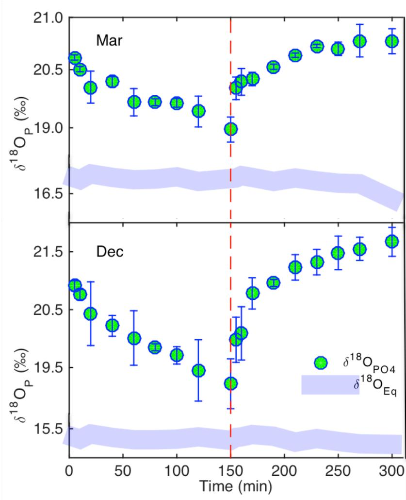
Figure 15 Phosphate oxygen isotope ratios of dissolved  $\text{PO}_4$  in the aeration basin of KCRWTF. The vertical red dashed line represents the switching of anoxic condition (by stopping aeration) and the purple light color zone represents the calculated equilibrium values. The upper and lower boundaries of the equilibrium zone is calculated based on equations 2 and 3 after Longinelli and Nuti, (1973) and Chang and Blake (2015), respectively.
