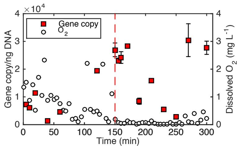
Figure 16 Copies of poly-P accumulating genes in activated sludge collected from KCRWTF.
