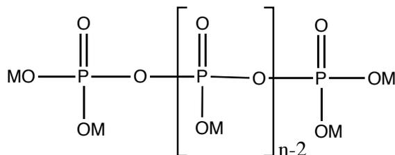
Figure 1 Structure of poly-P (of chain length  $n$ ). M represents a hydrogen or a monovalent metal cation.
