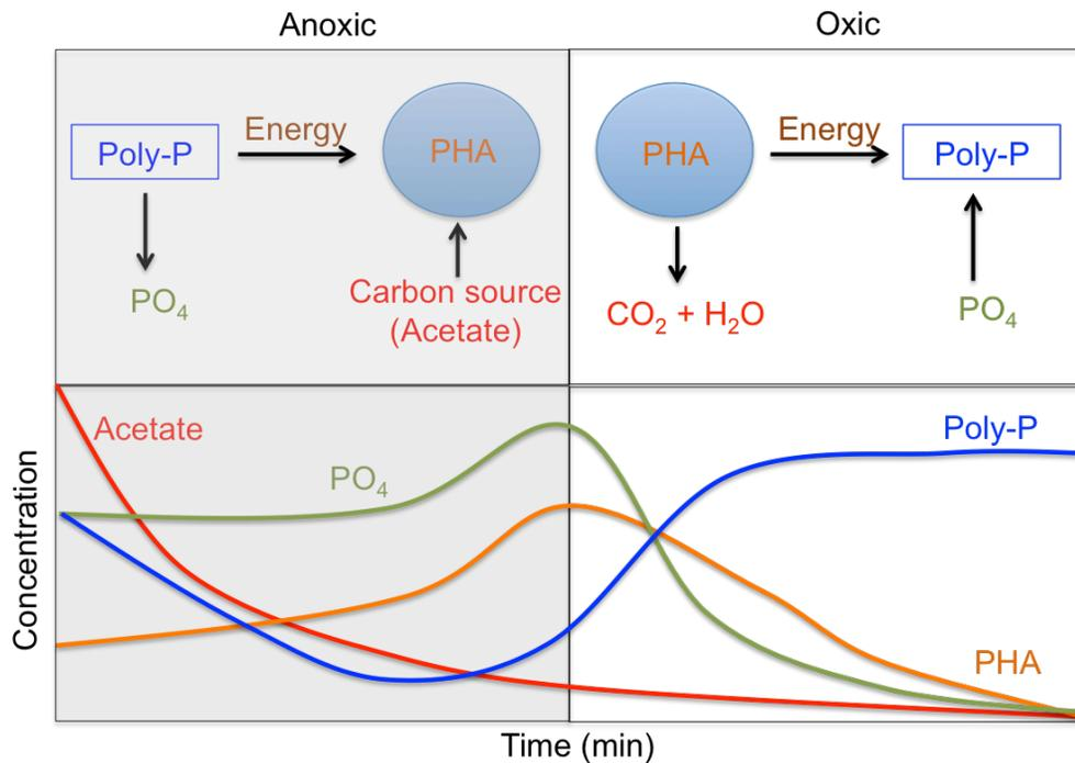
Figure 3 Trends of PHA, PO<sub>4</sub>, poly-P, and acetate concentrations during alternating anoxic and oxic cycles in EBPR process (re-drawn from Forbes et al., 2009).
