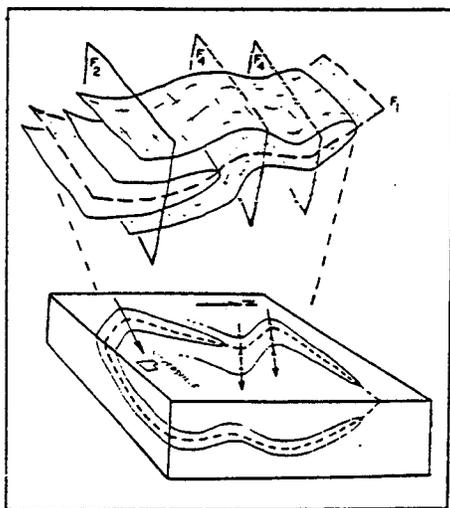
Fig. 16. Block diagram showing how interference between  $F_1$ ,  $F_2$ , and  $F_4$  fold sets produce the outcrop pattern of the  $F_1$  Canada Lake isocline. The axial plane of the  $F_1$  fold is stippled and its fold axis plunges 10-15° to the southeast. The city of Gloversville is shown.
