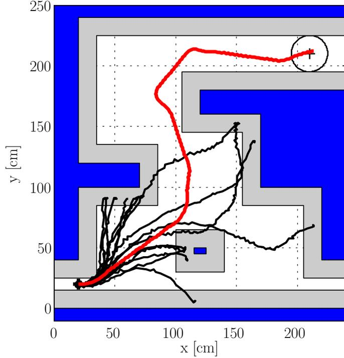
**Figure 3.18:** Experimental results with the OctoRoACH commanded to follow the desired trajectory generated by the RRT solver in open-loop.  $I = 15$  trials are considered. As expected by the simulations, open-loop execution of the desired trajectory is unsatisfactory. The robot collides with its environment soon after it starts navigating.
