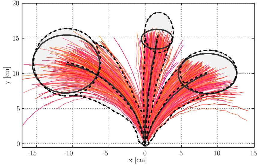
**Figure 4.3:** Output of the stochastic model, tuned according to the values in Tables 4.4 and 4.6. 248 random model instantiations are plotted over the experimental averages and cones of data. Similarly to Figure 4.2(b), model-predicted statistics follow closely the experimental statistics.
