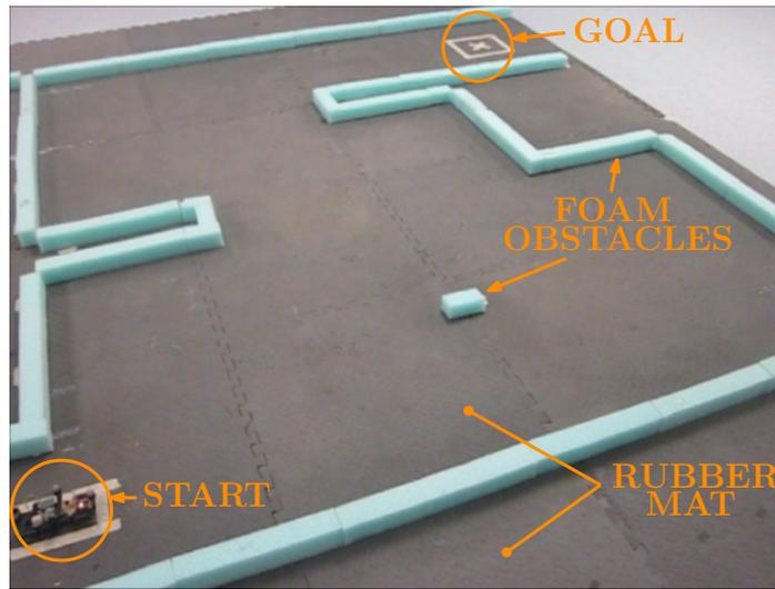
**Figure 3.16:** The physical environment realizing the case studies considered here. The robot starts at the bottom left corner and is required to navigate to the top right corner of the environment, while avoiding collisions.
