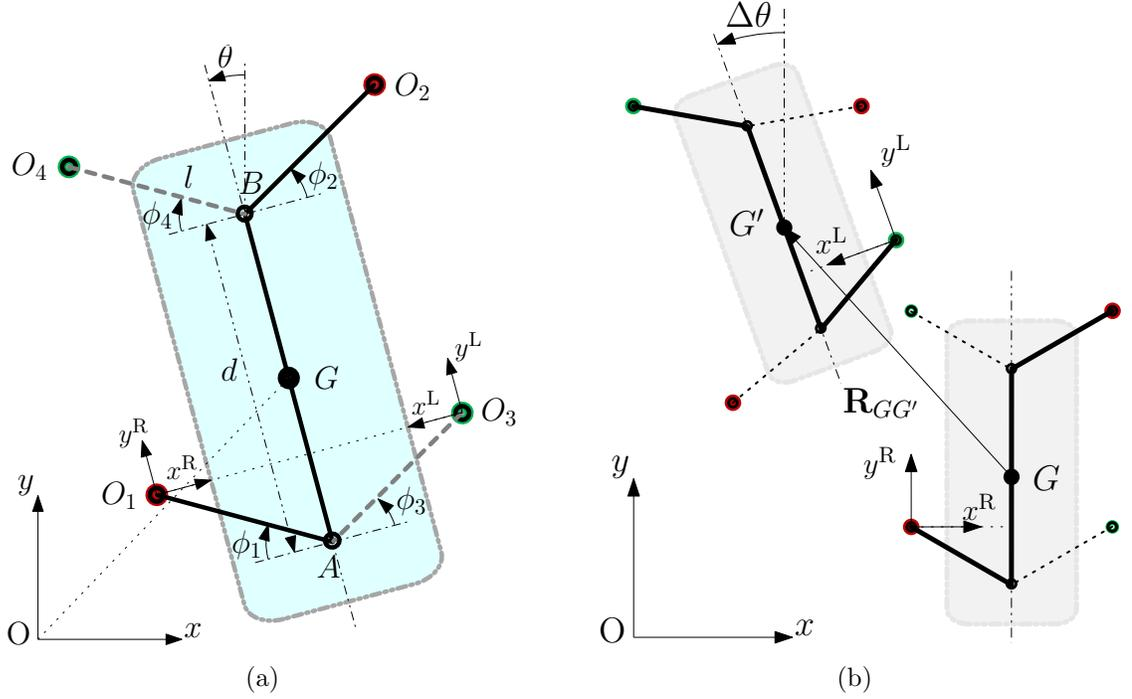
**Figure 3.1:** (a) The SFM template. Two pairs of rigid legs become active in turns, forming two fourbar linkages,  $\{O_1A, AB, BO_2\}$  and  $\{O_3A, AB, BO_4\}$ .  $d$  is the distance between the two hip-point joints  $A$  and  $B$ ,  $l$  denotes the leg length, and  $G$  is its geometric center. (b) Pictorial representation of state propagation—the active pair is marked with thick solid lines.
