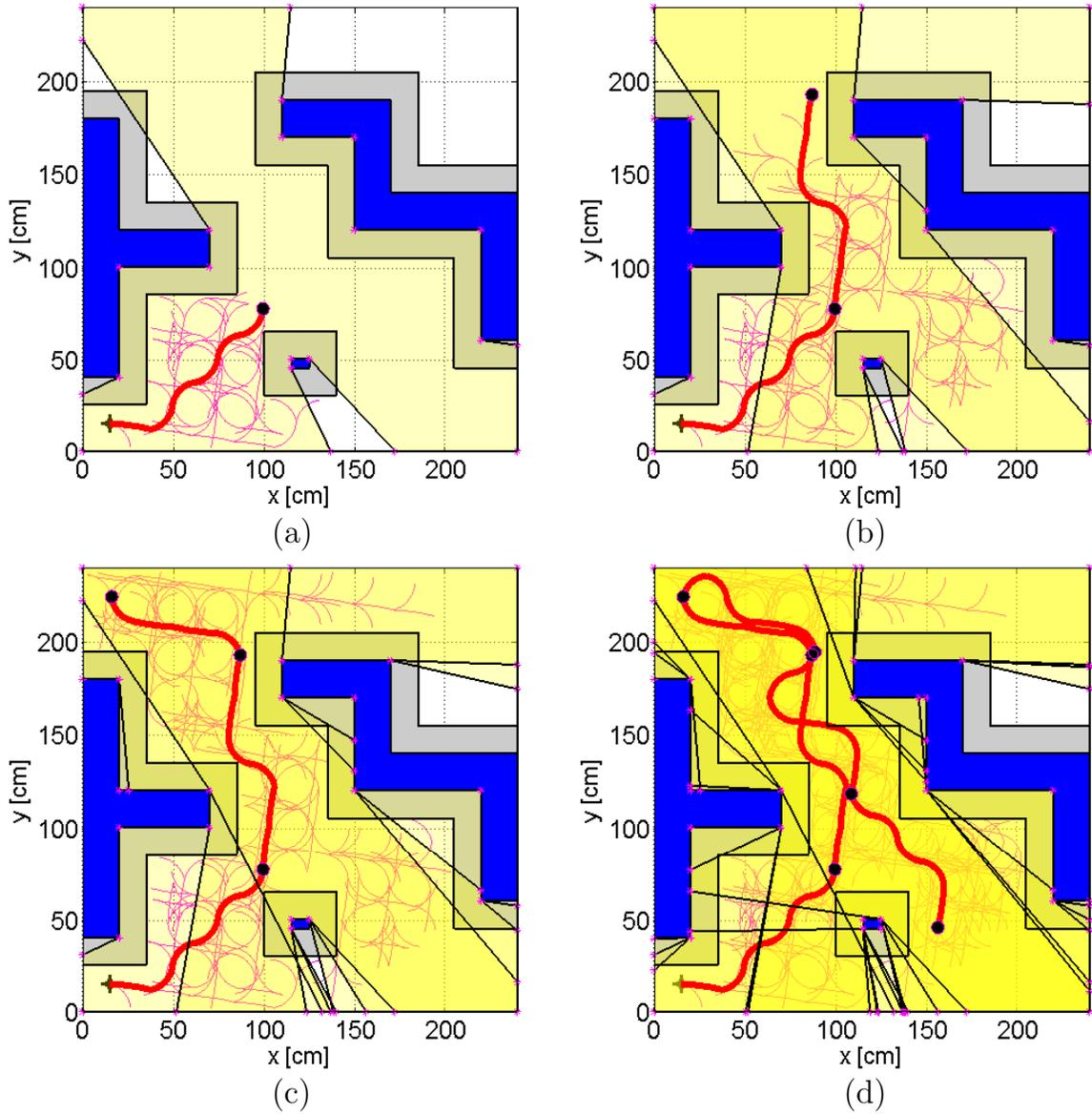
**Figure 3.25:** An example of a more complex task: surveillance under visibility-based and operational tempo constraints. Our approach works in a recursive fashion. (a) It first constructs a sub graph of the reachability tree (thin lines), and selects the node that maximizes the visibility polygon (highlighted region). (b)-(d) Then the system navigates to the selected node and the process repeats.
