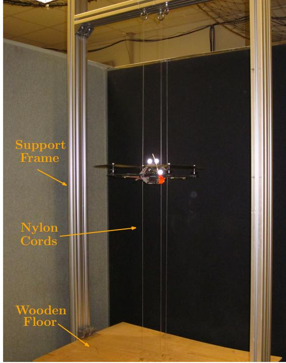
**Figure C.1:** The experimental setup. Our support structure aids in restraining the motion along the vertical direction only. The driving strings are composed of nylon cords; they provide strong support and minimal friction, while minimizing the fluctuations on the normal to the motion plane. We also added a wooden floor to artificially generate the ground effect.
