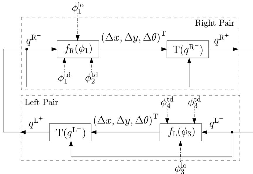
**Figure 3.2:** Model state propagation. State propagation in the local frame is mapped to the global frame through the homogeneous transformations  $T(q^{\text{R}^-})$  and  $T(q^{\text{L}^-})$  on  $\text{SE}(2)$ . Note that the end state of a pair is used directly to initiate the next one.
