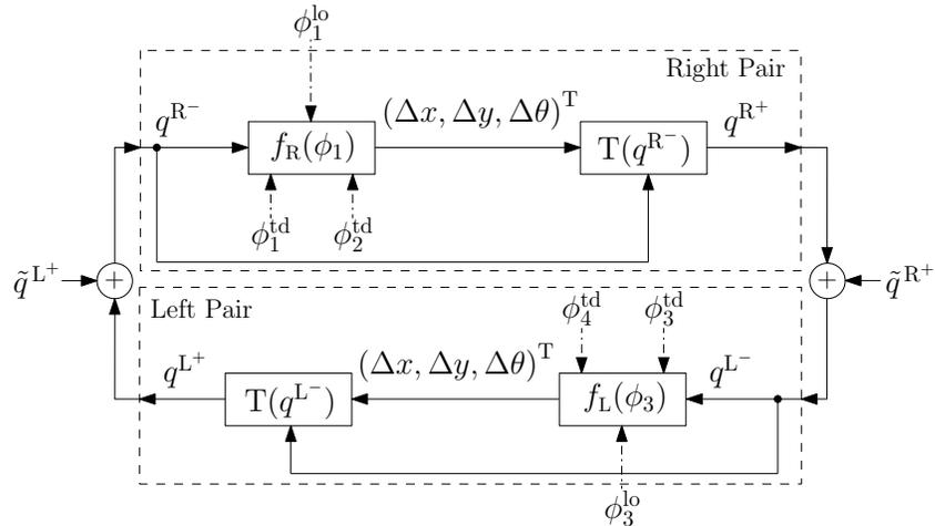
**Figure 3.19:** Model state propagation with injected step-by-step uncertainty. The uncertainty is added at a step's end state expressed in the global frame, and is  $\tilde{q}^{R+}$  for a right step or  $\tilde{q}^{L+}$  for a left step.
