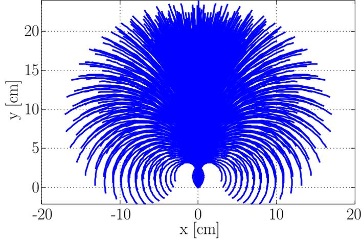
**Figure 3.8:** The set of reachable states produced by the SFM, starting at the initial state  $x_0 = (0, 0)$  cm,  $\theta_0 = 0^\circ$ , spanning 10 model steps. Not all possible combinations of touchdown and liftoff angles are shown; this leads to some small areas not being covered by the paths.
