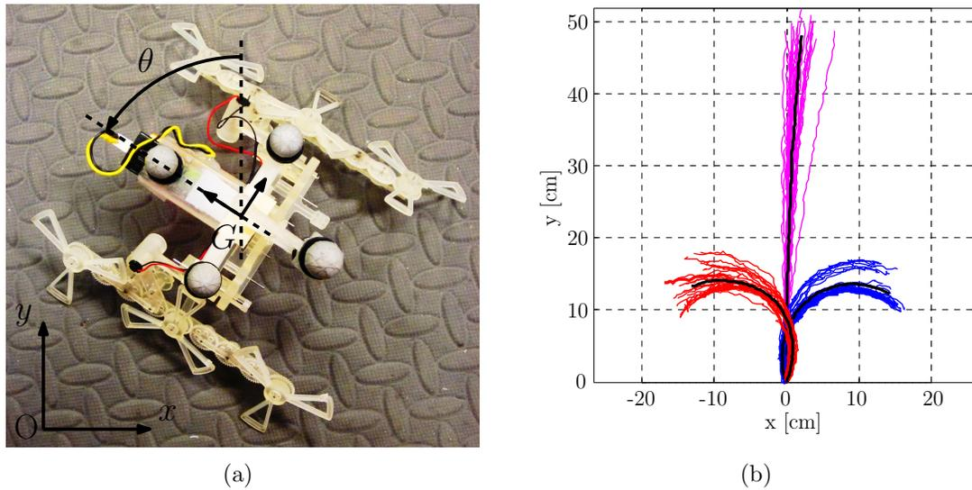
**Figure 3.26:** (a) The state of the robot is  $(x_G, y_G, \theta) \in \mathbb{R}^2 \times \mathbb{S}$ . (b) Data collected from STAR. Thin curves depict the evolution of the geometric center of the robot, while the experimental sample means out of a total of 30 paths for each case is shown in thick curves.
