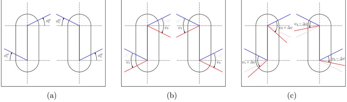
**Figure 3.3:** Model configurations to achieve straight-line and curved paths. (a) The initial configuration is determined by setting the touchdown angles,  $\phi_i^{td}, i = 1, \dots, 4$ . (b) Straight-line paths are achieved when the leg touchdown and liftoff angles are symmetric with respect to the horizontal body axis (equivalently, all sweep angles are equal). (c) Creating asymmetry,  $\Delta\psi$ , in the sweep angles enables turning of the model.
