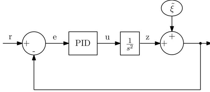
**Figure C.4:** Schematic representation of the modified closed-loop control architecture. As before, the input  $r$  denotes the desired hovering height, and the PID gains have been tuned a-priori.
