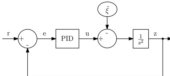
**Figure C.3:** Schematic representation of the closed-loop control stochastic model for the steady-state vertical dynamics component during quadrotor hovering. The input  $r$  denotes the desired hovering height, while the gains of the PID controller have been tuned a-priori, and remain the same with those used in our data collections. In  $\tilde{\xi} \sim \mathcal{N}(0, \sigma_\xi^2)$ , the variance  $\sigma_\xi^2$  is estimated using the proposed algorithm.
