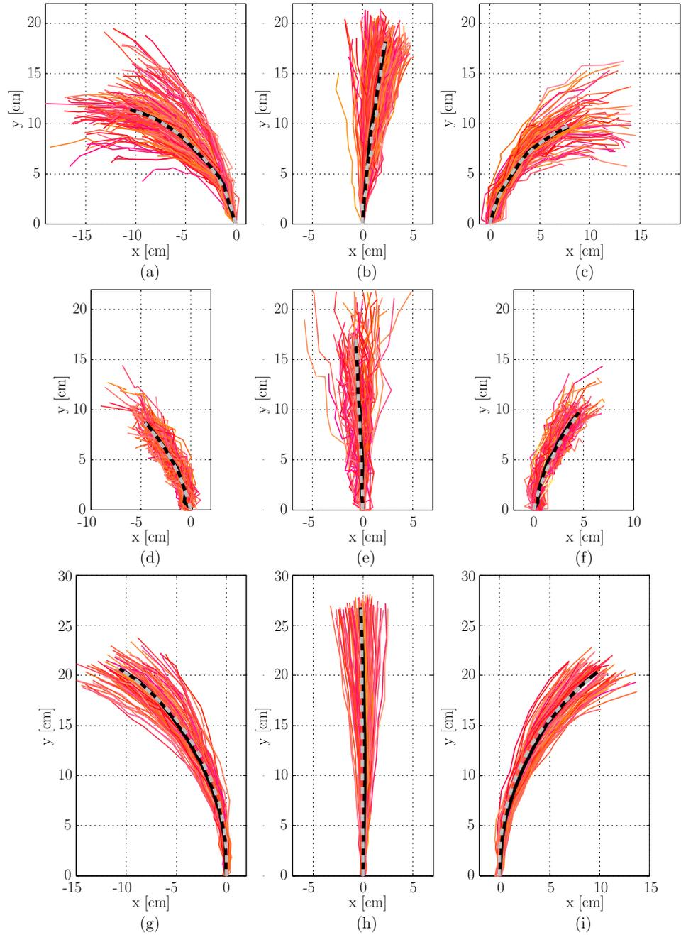
**Figure 3.14:** Experimental data for the motion primitives considered here. Individual paths are shown with thin curves, while experimental averages are marked with thick curves. The SFM outputs that capture best these experimental averages are shown with lightly-shaded dashed curves. (a)-(c) CCW, SL, and CW primitives for the OctoRoACH. Similarly (d)-(f) for the revamped OctoRoACH, and (g)-(i) SPIDAR.
