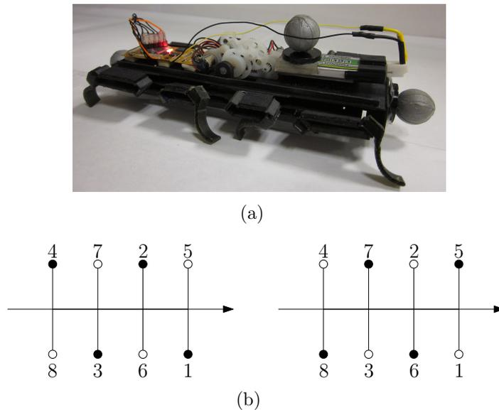
**Figure 3.9:** (a) The OctoROACH [120] designed and manufactured at the University of California, Berkeley. Its body size is 130x60x30 mm, it weighs 35 g, and it can reach a maximum speed of 0.5 m/s.(b) The foot-fall pattern of the robot, which results to an alternating tetrapod gait.
