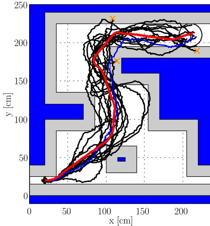
**Figure 3.22:** Experimental results with the OctoRoACH. As before, the desired trajectory is marked with a thick curve (in red), and we repeat the trial for 15 times. The combination of local trajectory tracking control with the prediction phase enables the robot to successfully complete its task most of the times (terminal collisions are marked with a cross).
