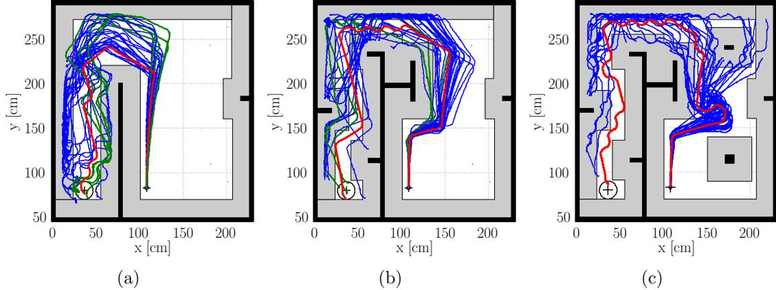
**Figure 3.28:** Experimental implementation of the plans shown in Figure 3.27. (a) Least complex workspace: 4 paths (in green) reach the desired configuration. (b) Medium-complexity workspace: 3 trials reached the goal. (c) No successful trials were recorded for the hardest workspace.
