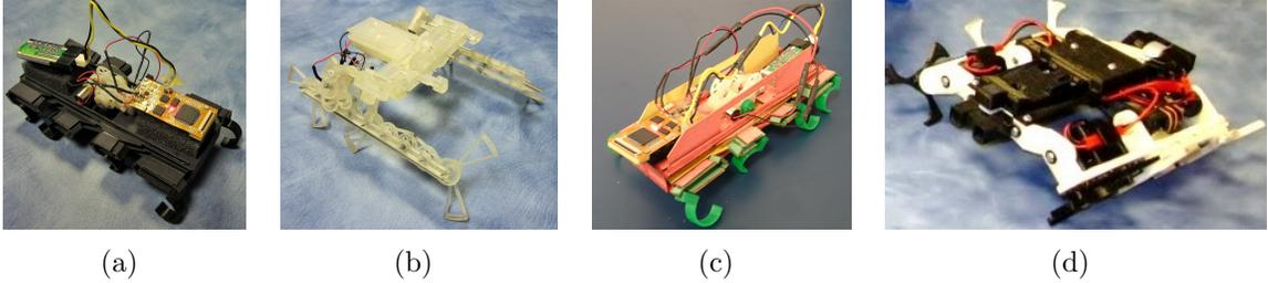
**Figure 1.4:** A family of miniature legged robots studied in this work. (a) The eight-legged OctoRoACH [120], and (b) the 3D-printed STAR [161]. Both robots are designed and manufactured at University of California, Berkeley. Inspired by these designs, we redesigned and manufactured in-house (c) a revamped OctoRoACH able to carry more payload, and (d) SPIDAR, a heavy-duty, highly-versatile miniature legged robot.
