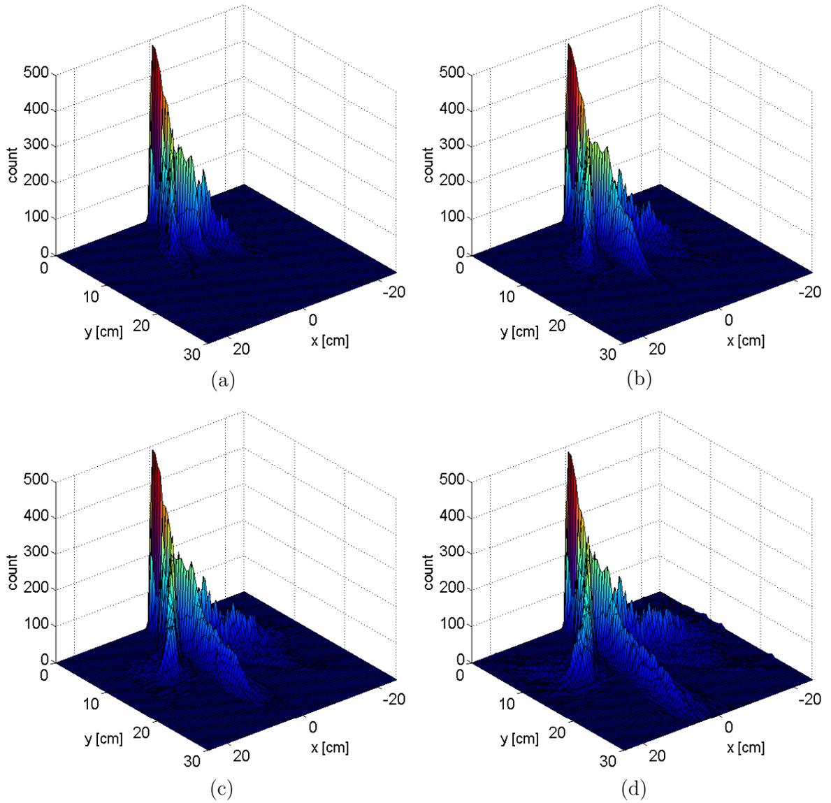
**Figure 3.13:** Path dispersion at (a) 2 sec, (b) 2.5 sec, (c) 3 sec, (d) 3.5 sec for the OctoRoACH. All primitives start at the origin, and are largely dispersed at the end of the 3 sec trial as shown in (c). The  $z$  axis counts the number of paths that are inside a particular grid square. Due to the selected grid size, some paths may appear more than once inside a square.
