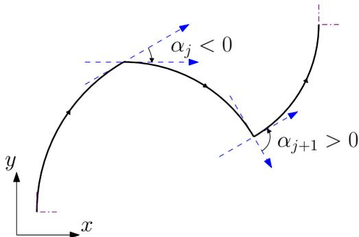
**Figure 3.7:** Instantaneous change in orientation when switching between steps. By convention, the sign of the angle is given by the right hand rule.
