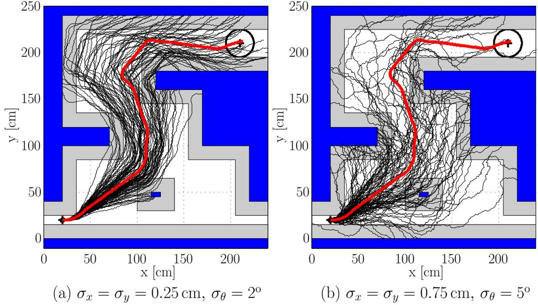
**Figure 3.17:** Simulated response of the system commanded to follow the desired trajectory shown earlier in Figure 3.15(a) (thick red curve), when uncertainty perturbs its state at the end of every step. In all cases we simulate 100 trials. (a) Open-loop response of the system with low magnitude of infused uncertainty scores a 10% success rate. (b) As the magnitude of the infused uncertainty grows, the system loses track of the desired trajectory, and the success rate reduces to 2%.
