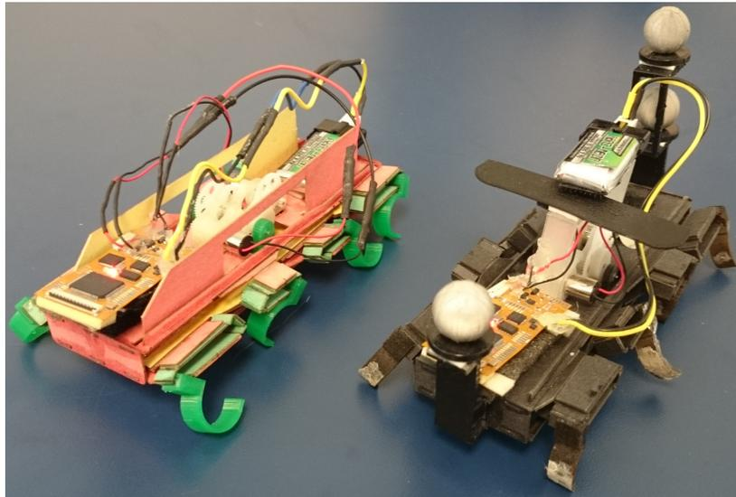
**Figure 3.11:** The revamped OctoRoACH compared to the original design. Under minimal modifications (described in text), the revamped OctoRoACH has improved durability, longer life-cycle, and increased payload capacity.
