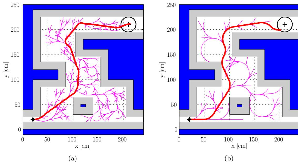
**Figure 3.15:** The RRT is combined with the motion primitives generated by the SFM template for the (a) OctoRoACH and (b) SPIDAR (see Table 3.2). The solver generates desired trajectories (thick curves) in environments populated with obstacles. We discard any edges and vertices that cross the boundaries of the augmented obstacle regions (lightly shaded areas) surrounding the actual obstacles (in blue).
