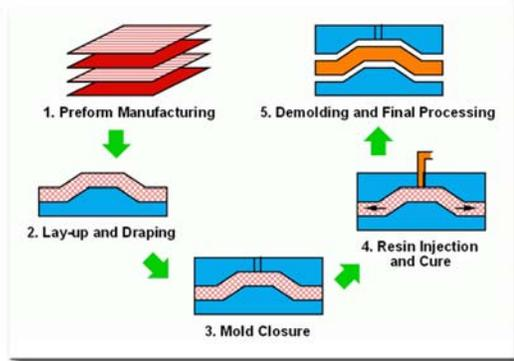
mold is closed and the resin is injected into the cavity under pressure. Once the liquid resin fills the mold cavity, it cures, during which the resin hardens due to the formation of polymeric network forming the matrix of the composite, allowing the part to be de-molded. Note that the mold walls are considered rigid and preform is stationary during the injection. This technique is well known and has been traditionally applied to moderately large parts in various
