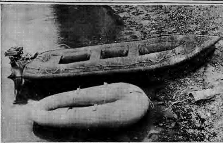
Two of the many types of boats that are being turned out by the rubber industry for use of the military forces are shown above. Products of The General Tire & Rubber Company, the small boat in the foreground is a parachute boat, used by pilots shot down over the water. The boat is attached to the pilot's chute and is inflated after he has dropped into the water. The other is a landing boat used by the Navy. In similar boats the Marines invaded the Solomon Islands.
