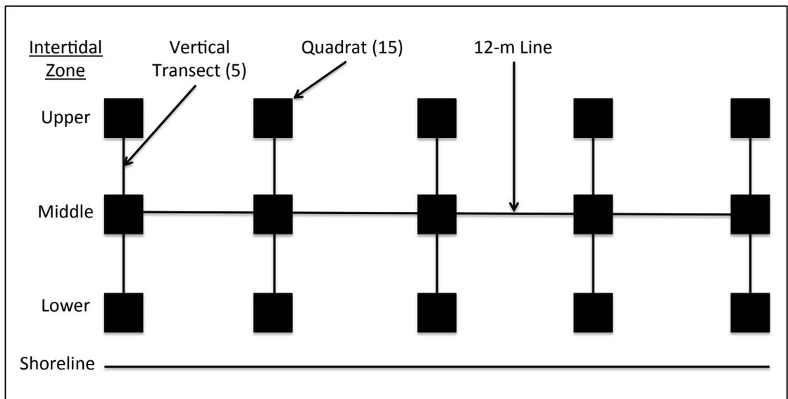
Figure 2.2: Vertical Benthic Sampling Design. Filled boxes show the location of sampling sites in upper, middle, and lower intertidal zones. Mean low-water shoreline is shown as a horizontal line at the bottom of the figure.
