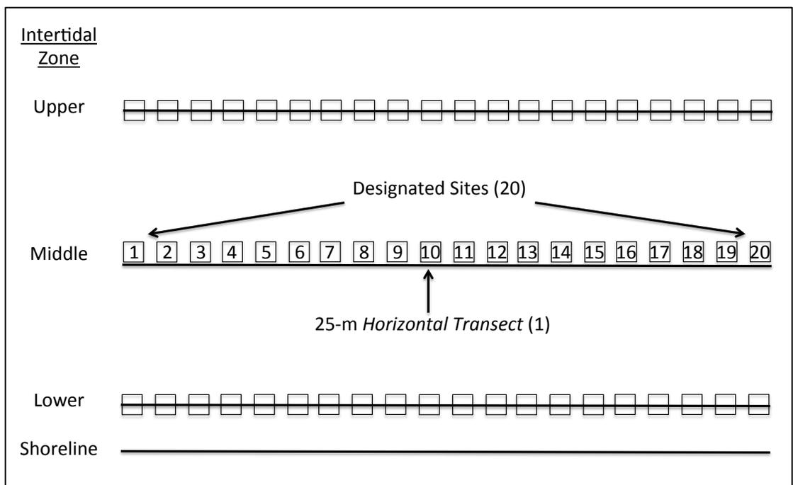
Figure 2.1: Horizontal Benthic Sampling Design. Numbered boxes show the arrangement of sampling locations in the middle intertidal zone. Open boxes show corresponding locations in the upper and lower intertidal zones. Mean low-water shoreline is shown as a horizontal line at the bottom of the figure. Sampling was restricted to the middle intertidal zone.
