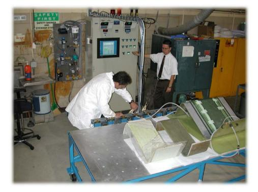
The infusion station includes: valves for on/off flow control of infusion lines, variable vacuum control, tool-mounted sensors, flow rate monitoring and temperature control of heated tooling. The software enables operator login, automated leak check, automated resin mixing, and automated infusion of large-scale and thick-section composite parts. All process variables and sensor information are stored in the QC database.
