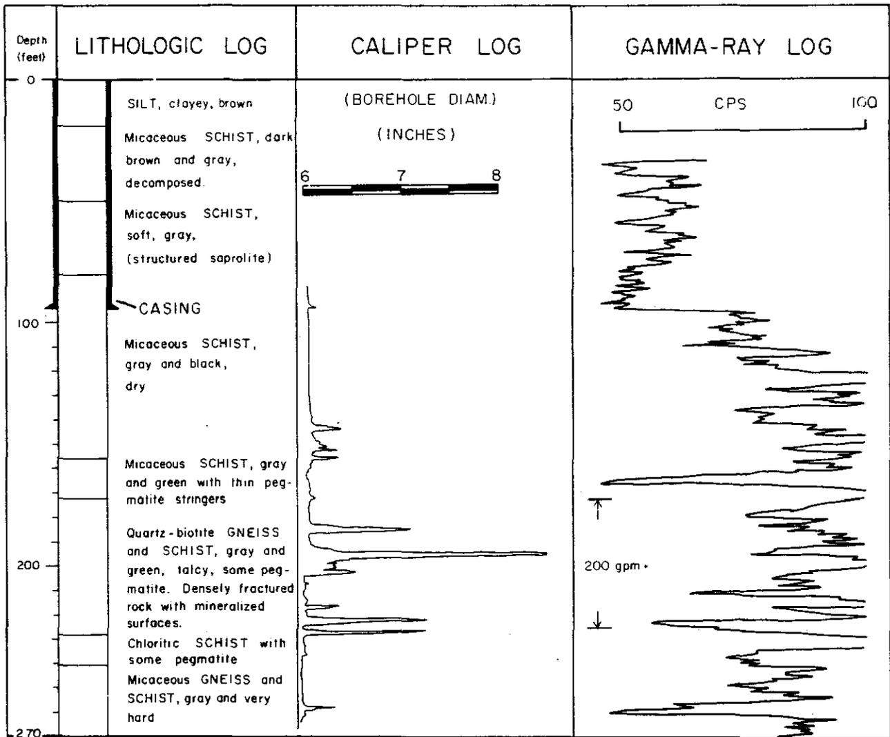
Figure 2. Lithologic, caliper, and gamma-ray logs of well Ca45-39 (After Talley, 1974).
