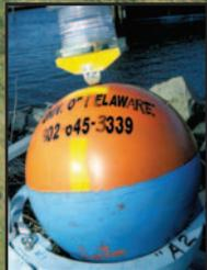
▲ This small buoy, or float, in Delaware Bay will mark the location of an Acoustic Doppler Current Profiler (ADCP), which measures the speed and direction of the currents.
