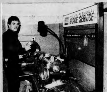
The new Ammco Brake Lathe, demonstrated by Ron Arches, Manager, is used in servicing of the brake system, including the turning of the brake drums and rotors.
