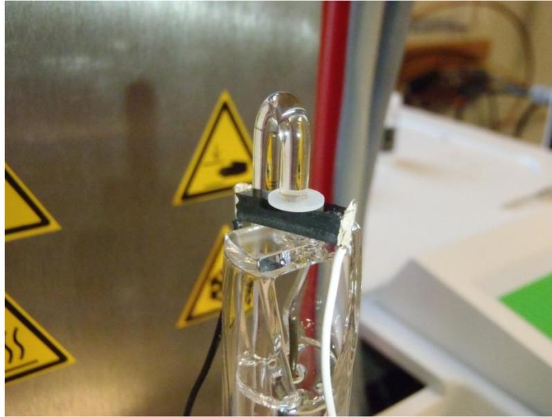
Figure 3.1: Photograph of nanocomposite specimen mounted on the TMA stage for thermoresistive characterization.
