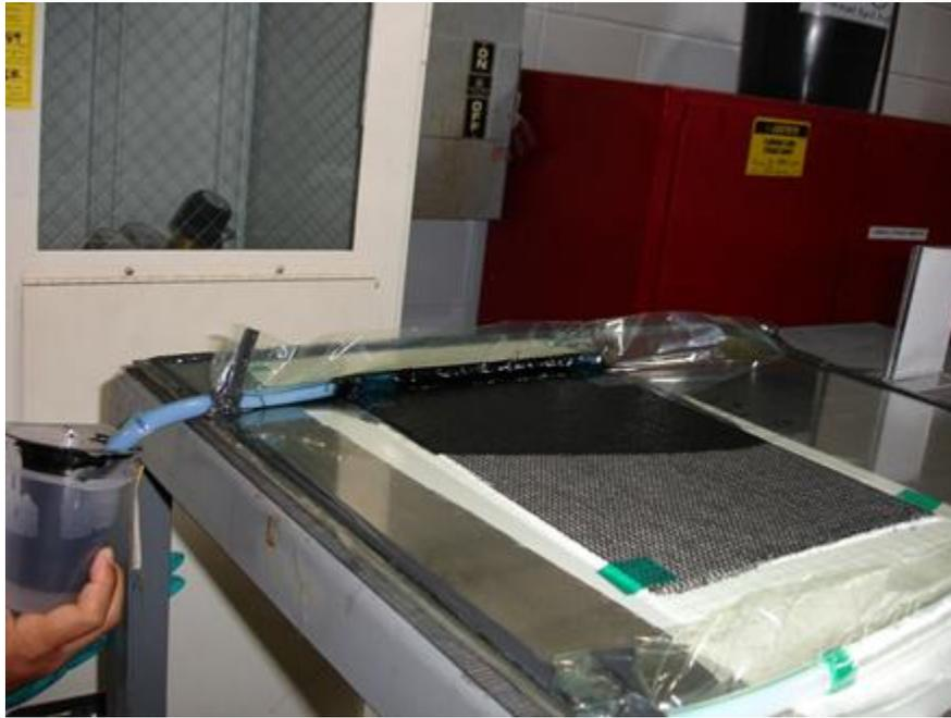
Figure 2.5: Photograph of glass fiber preform being infused with vinyl ester resin with dispersed CNTs. Used with permission of E.T. Thostenson.
