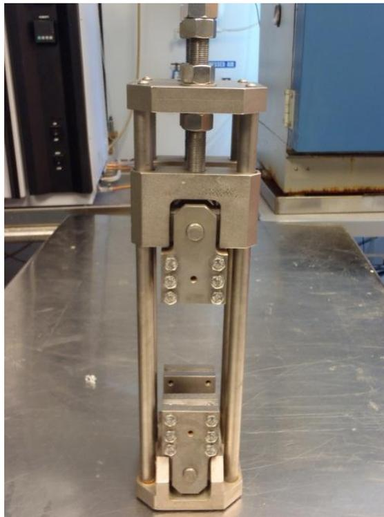
Figure 3.3: Constant displacement weathering fixture used for environmental testing of composites.
