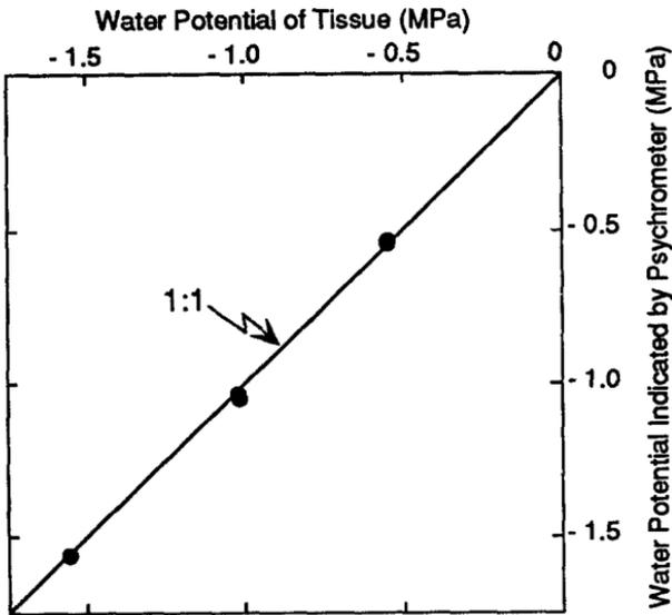
**Figure 3.7.** Test of the absolute accuracy of an isopiestic psychrometer. Water potential was measured with the psychrometer and compared with the known water potential for the same tissue. The known water potential was achieved by equilibrating the sunflower leaf tissue with an atmosphere of known water potential. Some replicate data points lie too close to one another to be resolved in this plot. From Boyer (1966).
