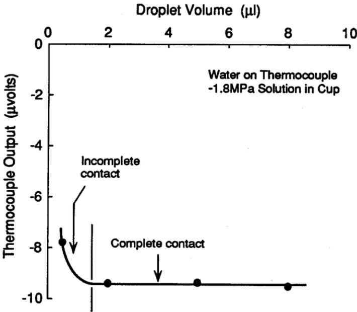
Figure 3.29. Effect of droplet size on thermocouple output. Measurements were made with an isopiestic thermocouple that completely contacted the droplet except when the droplet volume was decreased to 0.5  $\mu\text{l}$ .
