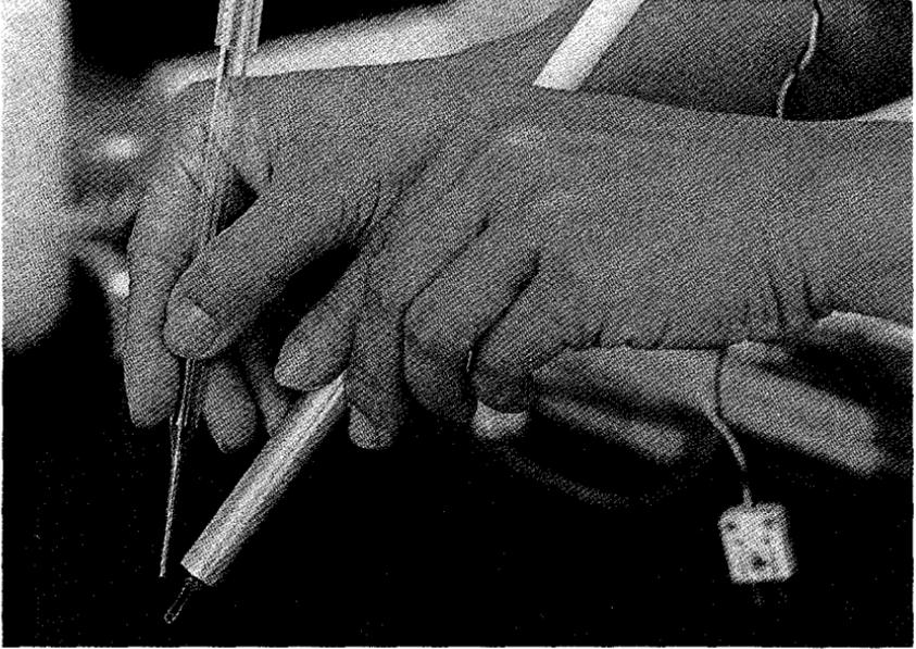
**Figure 3.9.** Drying the thermocouple from an isopiestic psychrometer in an air stream after rinsing the junction with water. Thermocouple and air stream should be directed downward to move water droplets away from the thermocouple.
