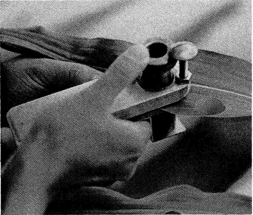
**Figure 3.13.** Cutting a tissue sample with a leaf punch and loading the psychrometer cup. Work swiftly to avoid sample dehydration.
