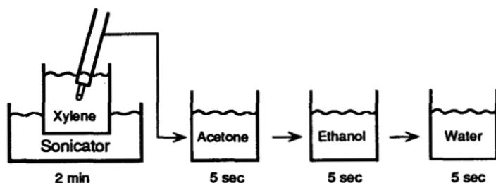
Figure 3.8. Cleaning a thermocouple from an isopiestic psychrometer.
