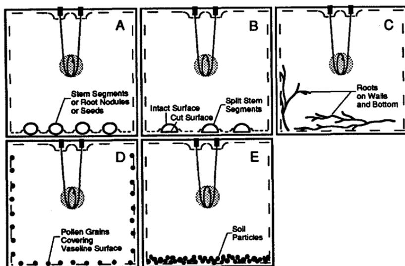
Figure 3.20. Placement of various plant parts or soil in the vapor chamber. A) Whole stem segments, root nodules, or seeds. B) Split segments of large stems. C) Roots. D) Pollen grains. E) Soil. Leaf placement is shown in Fig. 3.2.
