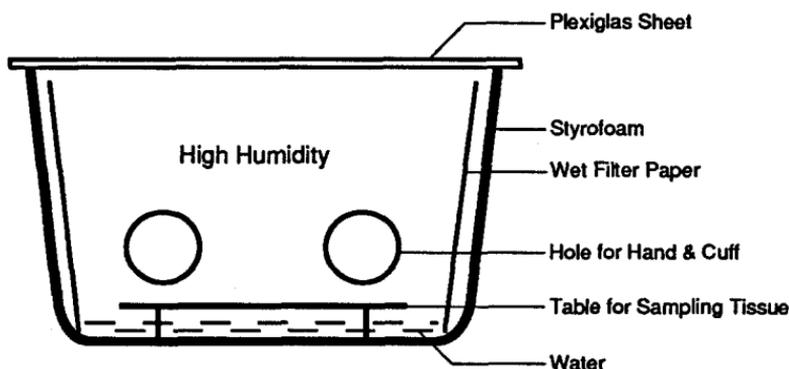
**Figure 3.32.** Glove box containing water-saturated air for sampling plant tissue and soils. The box has a clear top for viewing the sample on the table.
