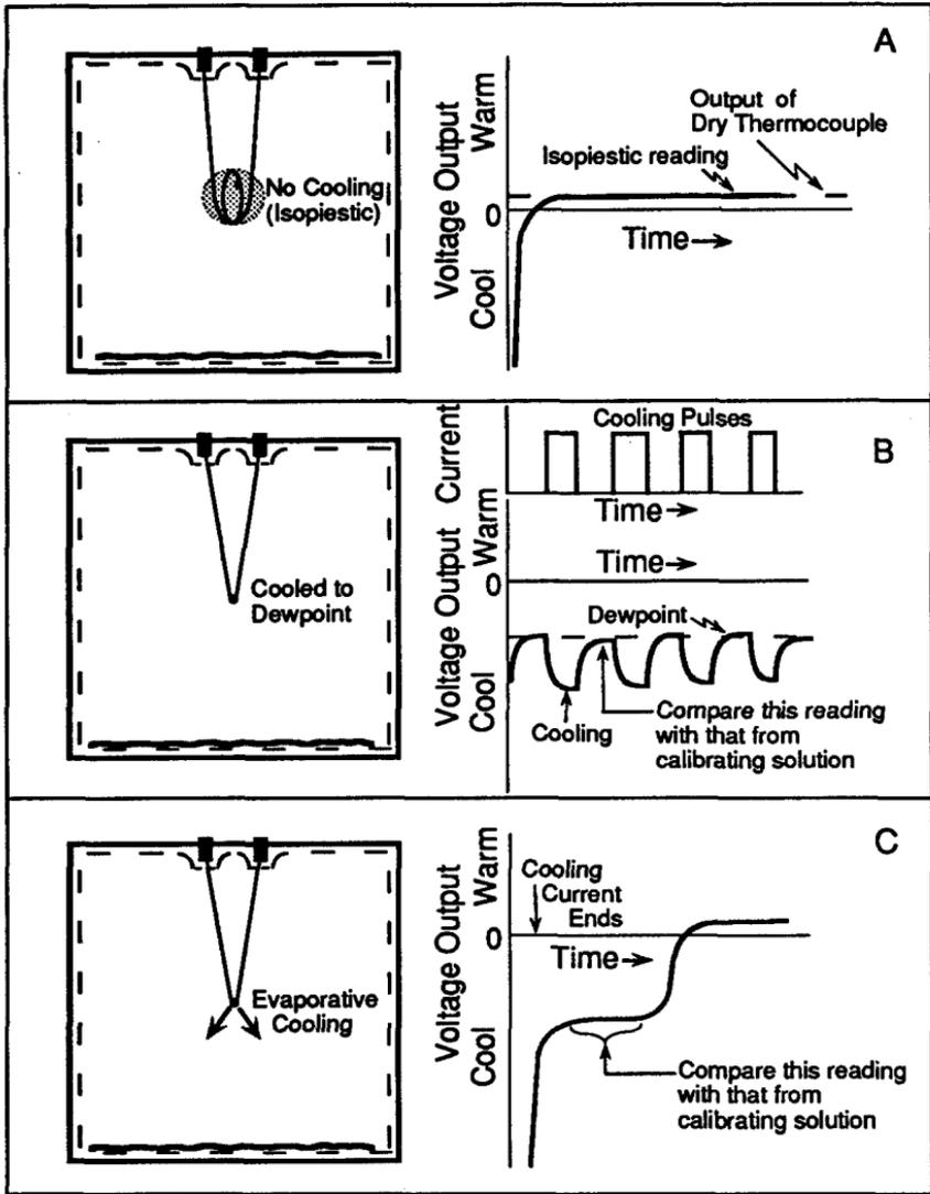
**Figure 3.6.** Three types of thermocouple psychrometers. A) Isopiestic psychrometer with a thermocouple that holds a droplet of solution of known vapor pressure (water potential). The thermocouple can be removed and the solution can be replaced with another having a different vapor pressure. The solution causing an output identical to that of the dry thermocouple is neither losing nor gaining water from the atmosphere and is thus isopiestic with the
