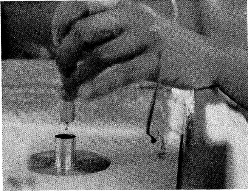
**Figure 3.16.** Inserting a thermocouple with new solution into a psychrometer system. Work swiftly to avoid dehydration of the droplet.
