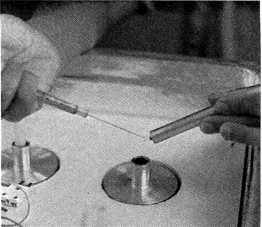
**Figure 3.15.** Replacing the solution on an isopiestic thermocouple. The droplet size has little effect on the thermocouple output (see Fig. 3.29).
