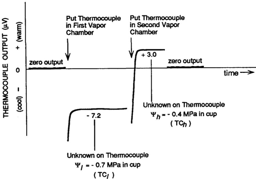
Figure 3.22. Recorder tracing of an isopiestic osmometer measurement. The isopiestic value is  $-0.49$  MPa, which is the osmotic potential needed in the cup to give a thermocouple reading of zero. See Eq. 3.7 for the calculation.
