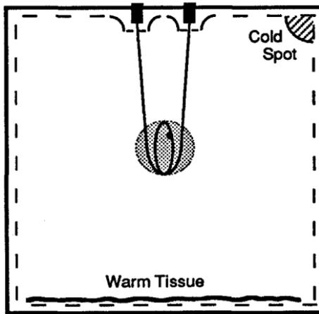
**Figure 3.30.** Effect of nonisothermal conditions (warm tissue or cold spots). External thermal gradients cause cold spots in the vapor chamber, resulting in condensation and disturbing the vapor conditions. Thermocouple readings cannot be corrected for these kinds of gradients. Internal gradients are caused by metabolic heat of the tissue. Measurements are corrected by noting the output of the thermocouple when dry and using the dry reading as the baseline for the output when wet.
