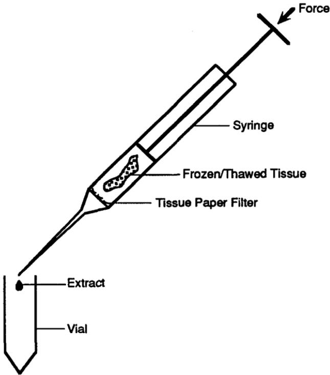
**Figure 3.23.** Extraction procedure after freezing and thawing plant tissue in the barrel of a syringe. Note tissue paper filter to prevent plant tissue from entering the syringe needle.
