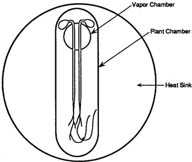
**Figure 3.21.** Example of a thermocouple psychrometer for measuring the water potential in intact plants. Etiolated seedlings are held in a plant chamber in a large aluminum heat sink. The vapor chamber for the psychrometer encloses the part of the plant to be measured. The vapor chamber is sealed around the stems with Vaseline.
