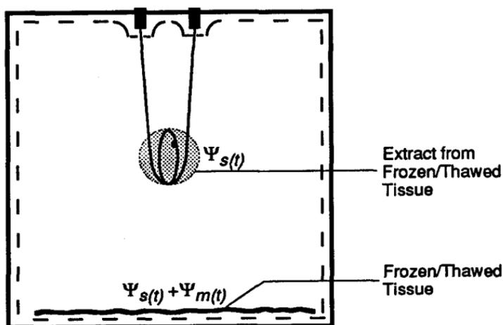
Figure 3.26. Measurement of matric potential in frozen/thawed tissue *in situ* ( $\Psi_m(t)$ ). The difference in potential between the frozen/thawed tissue ( $\Psi_s(t) + \Psi_m(t)$ ) and the osmotic potential ( $\Psi_s(t)$ ) extracted from a parallel sample is the  $\Psi_m(t)$  in the frozen/thawed tissue.
