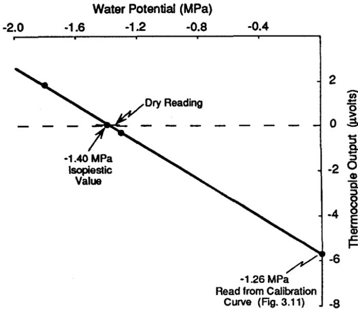
Figure 3.28. Diffusion error for a sample from a maize leaf. The true  $\Psi_w$  measured with the isopiestic psychrometer was -1.40 MPa while, with the same tissue sample, the same thermocouple measured only -1.26 MPa as a calibrated psychrometer (Richards and Ogata type) using the calibration curve in Fig. 3.11. Peltier psychrometers are subject to the same diffusion errors (Boyer and Knipling, 1965).
