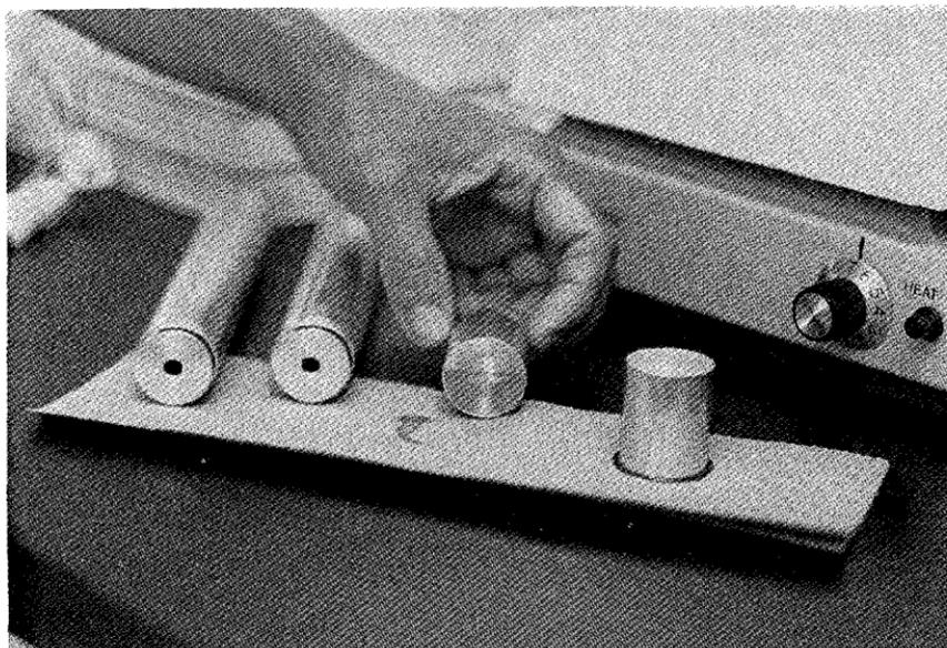
**Figure 3.10.** Coating the walls of a psychrometer cup with melted and resolidified Vaseline. The cup is cooled completely before reassembling the psychrometer. The chamber top, the walls of the entrance hole for the thermocouple, and the reference junctions of the thermocouple also are coated using unmelted Vaseline as in Fig. 3.5.
