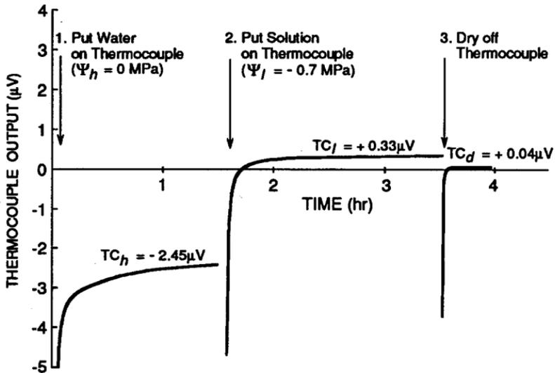
Figure 3.17. Recorder tracing of an isopiestic determination for a sunflower leaf. Measurement 1 gives a rough estimate of the water potential. Measurement 2 gives a more accurate estimate. The isopiestic value is the most accurate estimate and was  $-0.63$  MPa, calculated to give the output of  $TC_d$  (Fig. 3.18 and Eq. 3.2).
