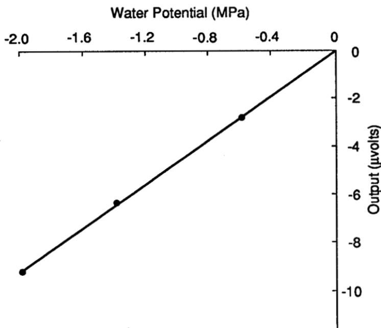
Figure 3.11. Typical calibration curve for Peltier or dew point psychrometer.
