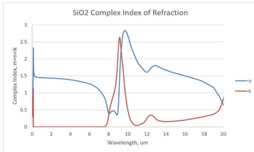
Figure 2.3: Complex index of refraction for Silicon Dioxide
