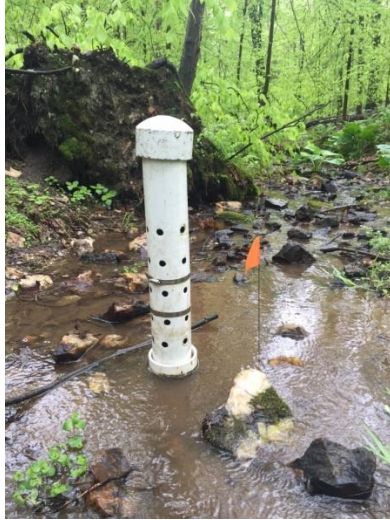
Figure 3.2: Photo of Composite Suspended Sampler (CSS) apparatus at baseflow conditions. Note orange flag for scale.
