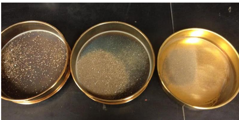
Figure 3.4: Sediment was sieved into three discrete size fractions using brass sieves. The percent weight for each size class was determined after sieving.
