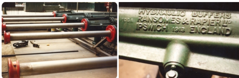
Fig. 10.3 English piston buffer system to stop runaway trains
