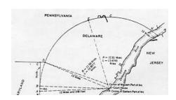
Lt. Col. J. D. Graham, U. S. Corps of Topographical Engineers, during the 1849 resurvey of the northeast corner of Maryland, correctly located the 12-mile distance in the area of the junction of the three states, creating the area known as "The Wedge".
