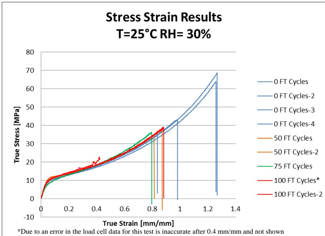
**Figure 9: Tensile Test Results at 25°C and 30%RH**
