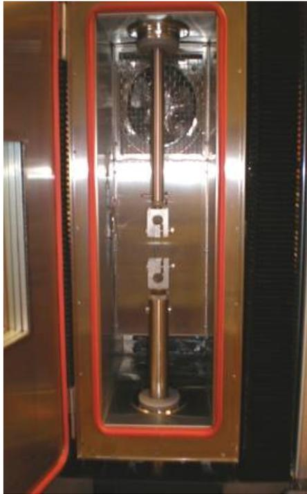
**Figure 6: Environmental Chamber Fitted with Materials Testing System**
