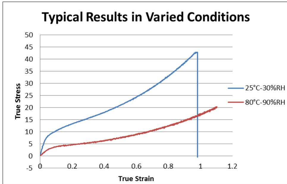
**Figure 3: Typical stress-strain results at two environmental conditions**
