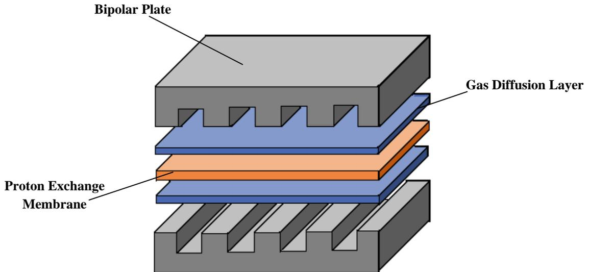
**Figure 2: Schematic of Stack Set-Up**
