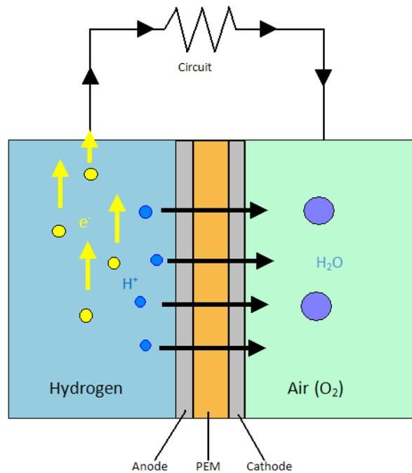
**Figure 1: Schematic of PEMFC reaction**
