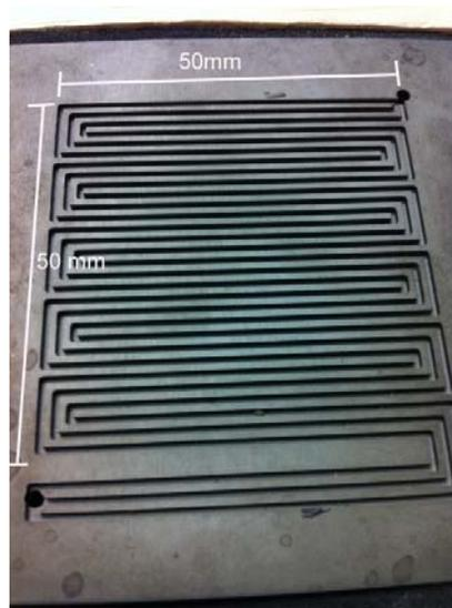
**Figure 4: Bipolar Plate**
