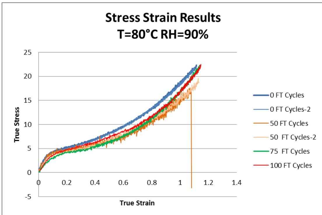
**Figure 10: Tensile Test Results at 80°C and 90%RH**
