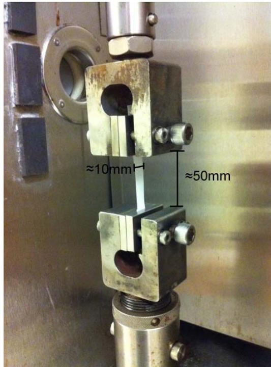
**Figure 7: Grips used for testing**
