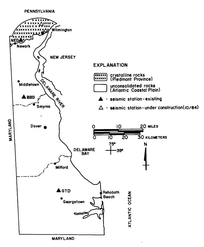
Figure 1. Map of Delaware Showing General Geology and Location of Seismic Stations.
