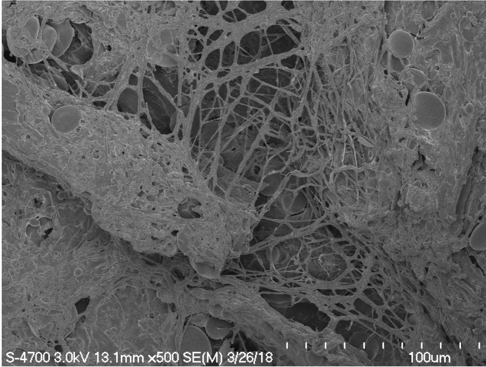
*Figure 3.* SEM image of reishi mycelium bonded with wood
