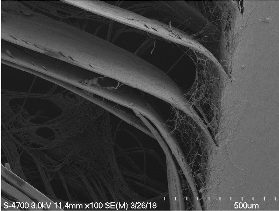
*Figure 5.* SEM image of reishi mycelium bonded with feather
