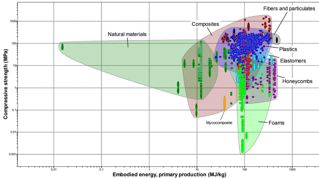
Figure 11. Comparison of materials on embodied energy and compressive strength
