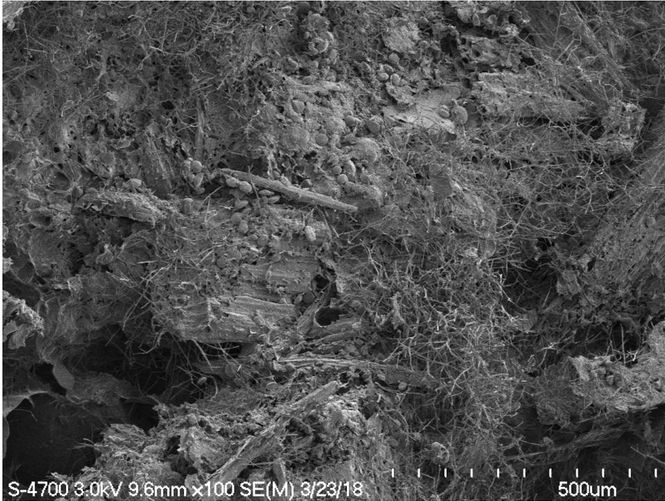
*Figure 4.* SEM image of king oyster mycelium bonded with wood
