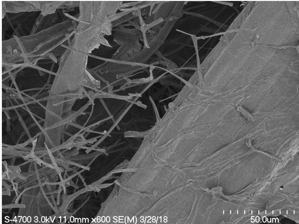
*Figure 7.* SEM image of king oyster mycelium bonded with fabric mat
