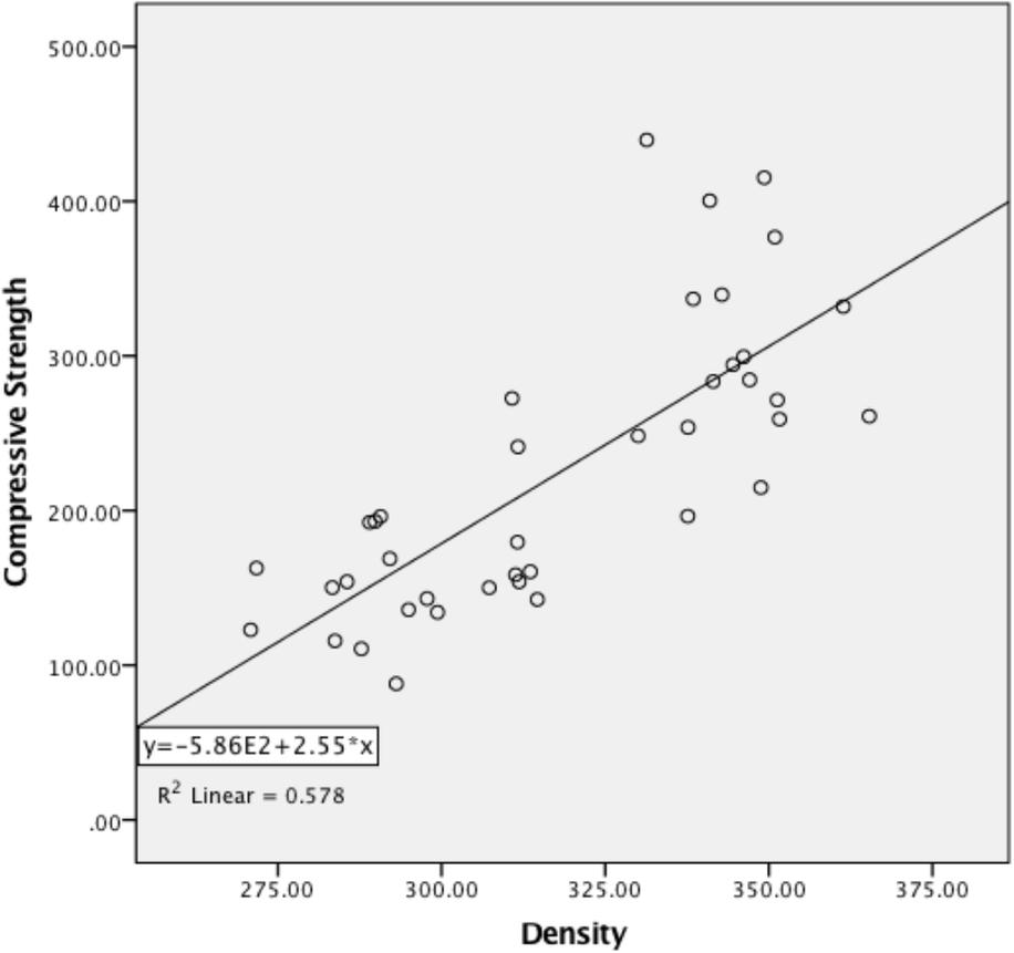
Figure 10. The relationship between density and compressive strength
