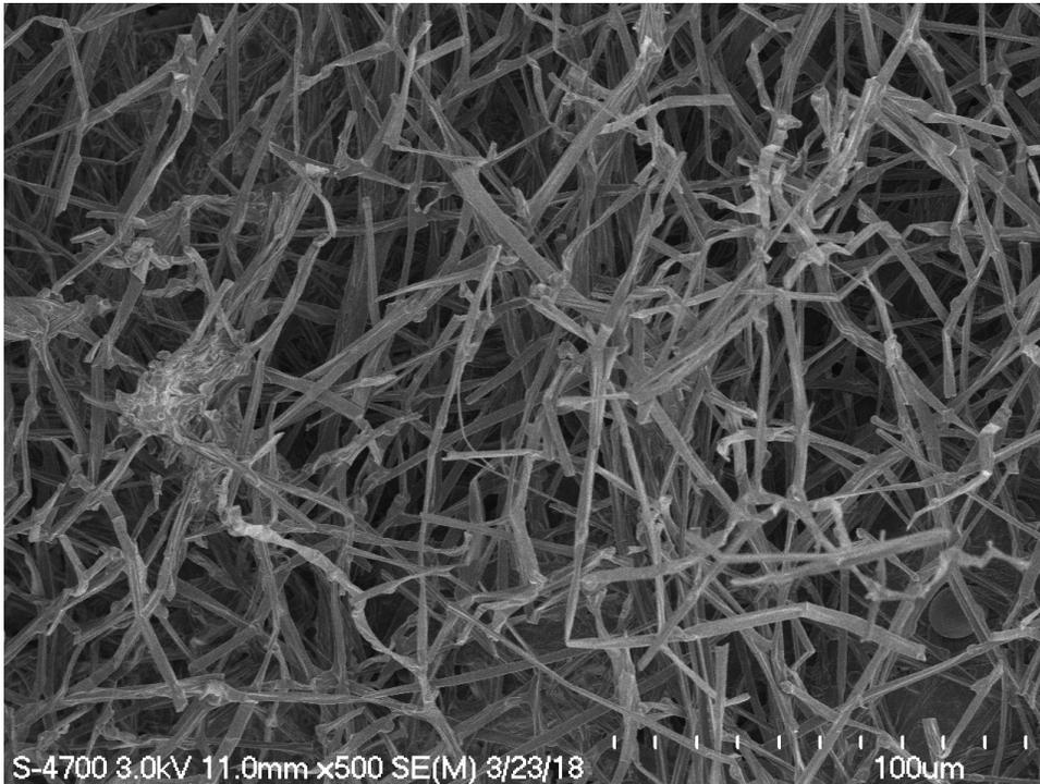
*Figure 2.* SEM image of king oyster mycelium matrix
