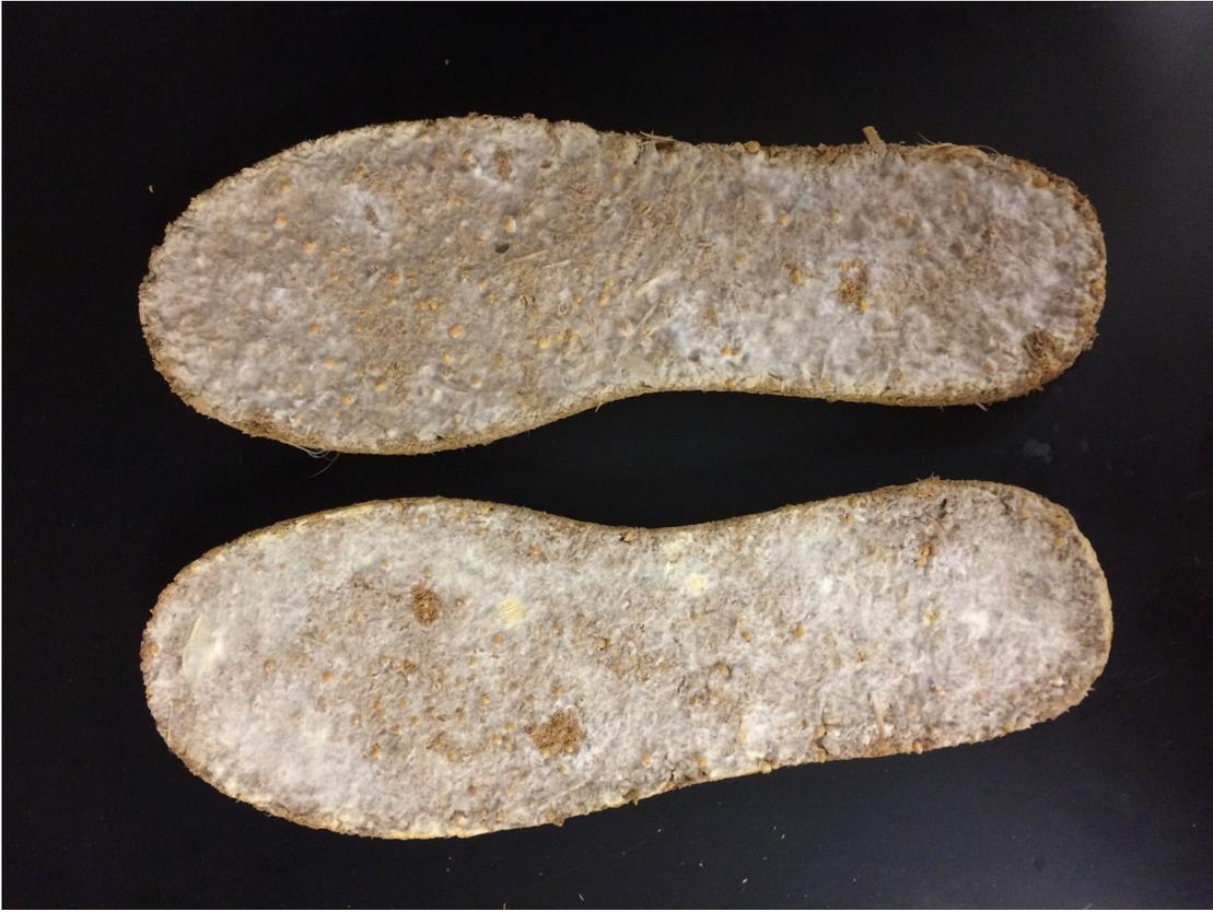
*Figure 12.* Mycelium shoe sole
