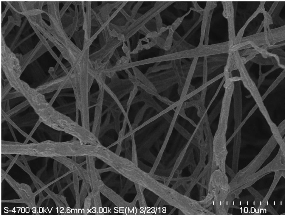
*Figure 1.* SEM image of reishi mycelium matrix
