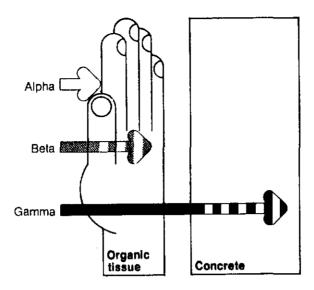
Figure 1. Examples of penetration abilities of different types of radioactive rays. (Source: U. S. Department of Energy, 1980).
