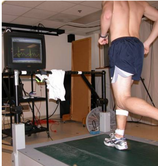
Figure 10: Example of real-time feedback from accelerometer presented to subjects while they ran on the treadmill.
