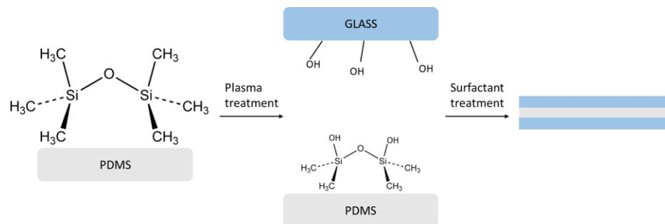
Figure 1.4: Example of the basic workflow to construct a sealed PDMS device. The hydrophilic silanol groups are exposed on the PDMS immediately after plasma treatment. After bonding, surfactants can be applied to further enhance hydrophilicity.
