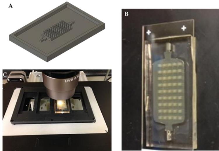
Figure 3.1: Representation of the components of the WormSlide and Big Brother assay system. (A) The WormSlide is produced from a 3D printed mold, which is then cast in PDMS. (B) The WormSlide is sealed between a glass coverslip and a glass coverslide, and has 45 individual wells and has a working volume of approximately 800  $\mu$ l. (C) The WormSlide is scanned using an automated translator, and imaging takes place on an inverted microscope.
