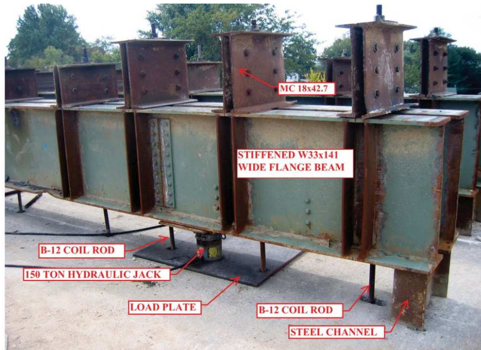
Figure 3.3 Photo of Loading Mechanism, Side View
