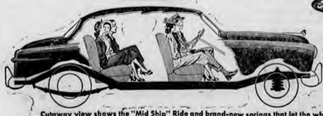
Cutaway view shows the "Mid Ship" Ride and brand-new springs that let the wheels
