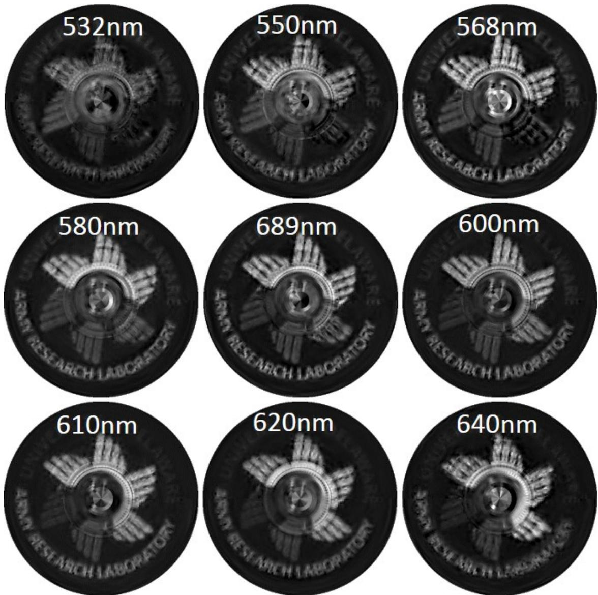
Figure 3.14: A total 16 spectral image bands are reconstructed from 64 low resolution measurements. The spectral range is from 500nm to 650nm. 9 of the 16 spectral bands are selected for display.
