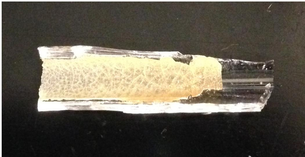
**Figure 3.5:** ZnO deposits in the entrance region of a reaction tube.
