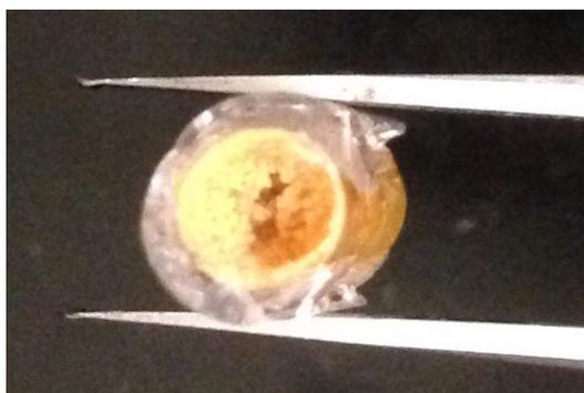
**Figure 3.7:** A reaction tube that is nearly clogged in the entrance region.
