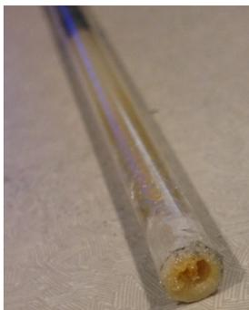
**Figure 3.6:** A reaction tube with significant ZnO deposition near the tube entrance.
