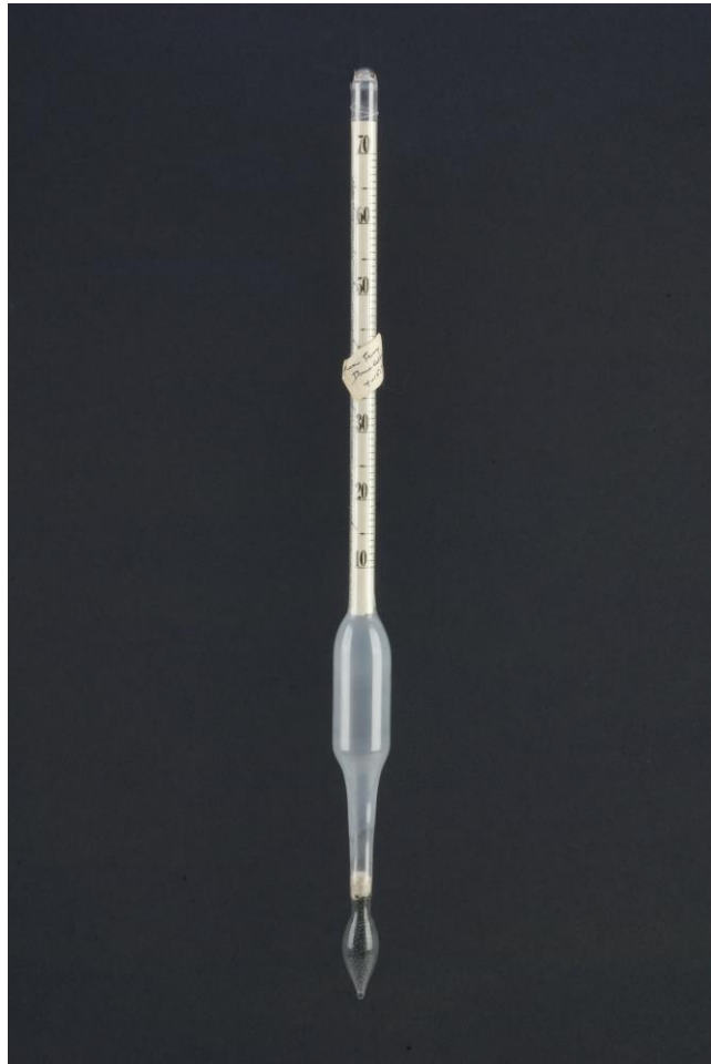
Figure 3.2 Beaume and Specific Gravity Scale for Light Liquids, possibly made by Jerry Donaldson, late 19 th – early 20 th century, United States or Germany. Glass, paper, lead. 10 \frac{3}{4} " x \frac{1}{2} ". Collection of Historical Scientific Instruments, Harvard University. Image Courtesy of Harvard University.
