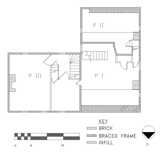
Figure 44: Reynolds House, second floor plan.
