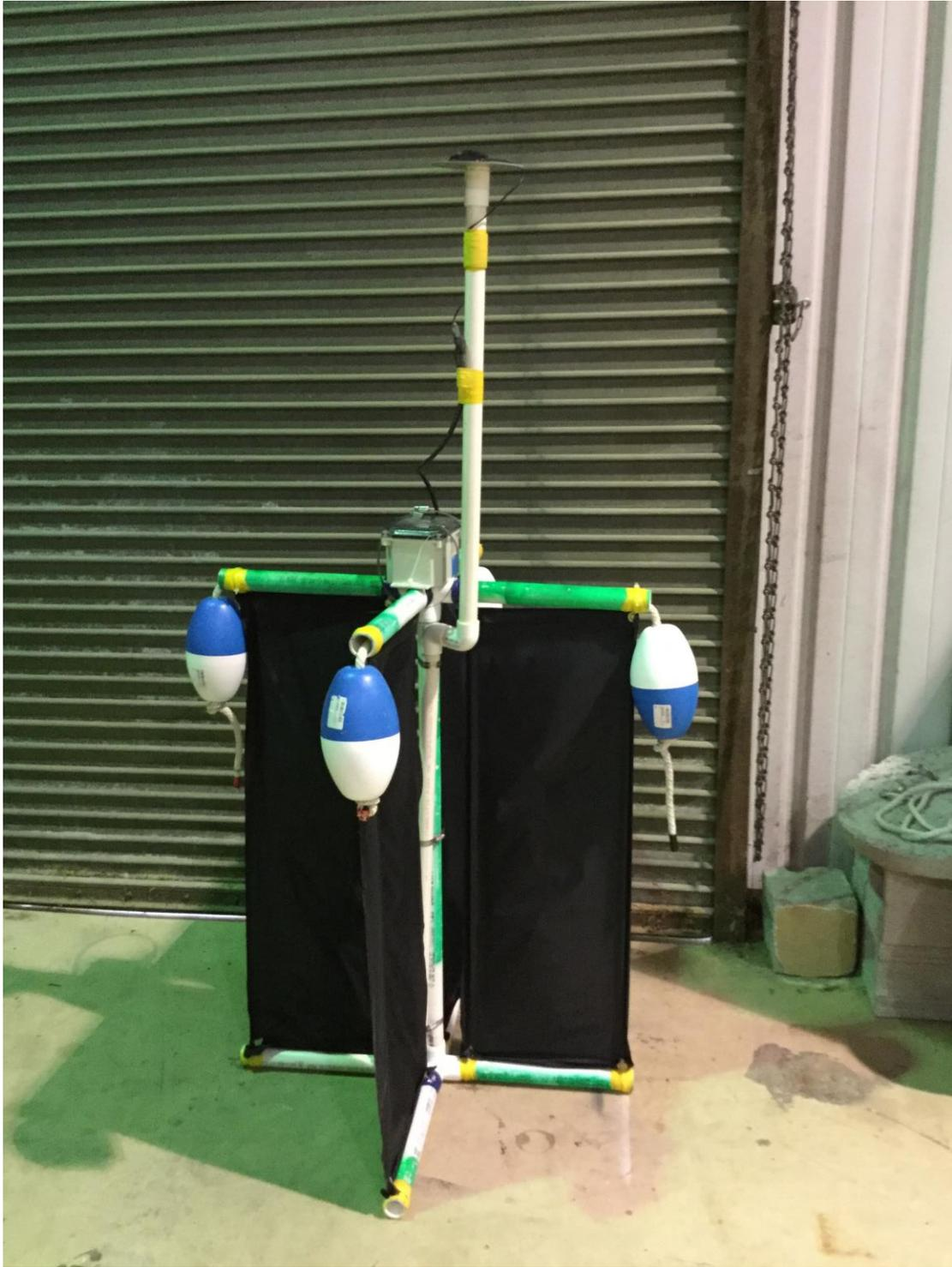
Figure 7: Wind slippage resistant drifter designed and constructed to investigate the impact of wind slippage on tracks from the primary drifters.
