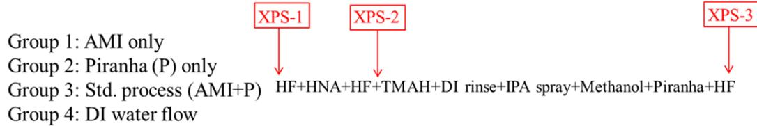
Figure 3.3: Processing sequence for the four batches of samples used for the wafer cleaning/texturing experiment [63].
