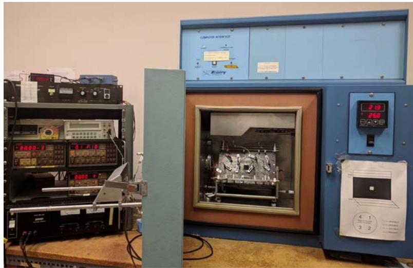
Figure 2.24: A Tenney Engineering Inc. enclosure for temperature dependent conductivity measurement, complete with a programmable electrometer, voltage source and channel scanner.
