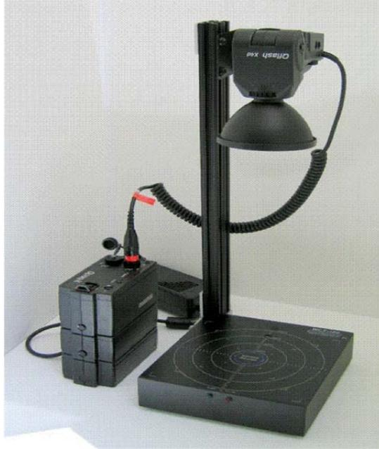
Figure 2.16: Sinton instrument WCT120 lifetime tester used for PCD and QSSPC measurement [58]
