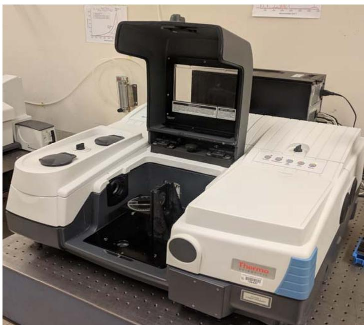
Figure 2.8: A FTIR Spectroscopy system by Thermo Scientific used for vibrational spectroscopic study.
