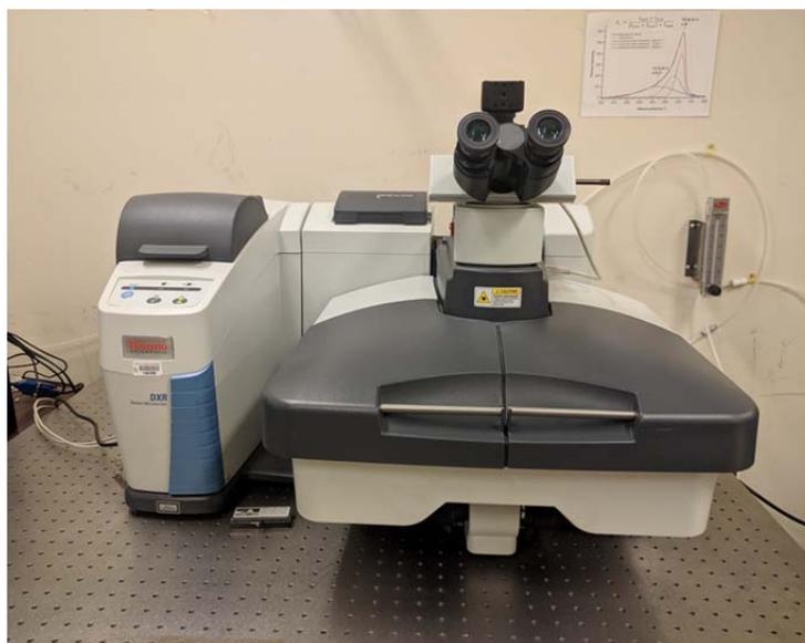
Figure 2.10: A Thermo Scientific DXR Raman Microscope complete with a 532 nm laser source used for Raman Spectroscopy.
