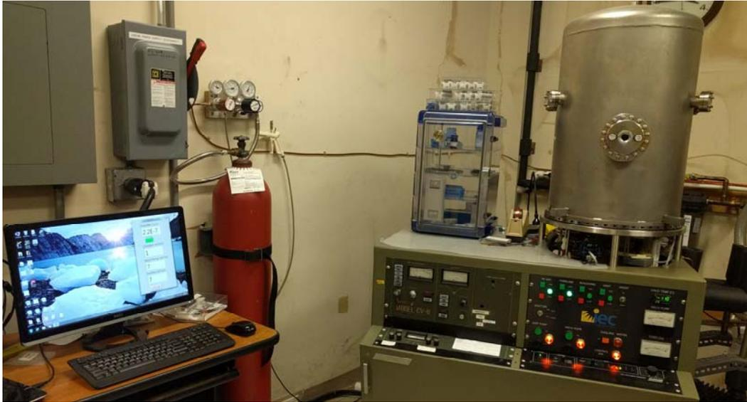
Figure 2.3: Electron beam (e-beam) evaporation system used for thin film metallization.
