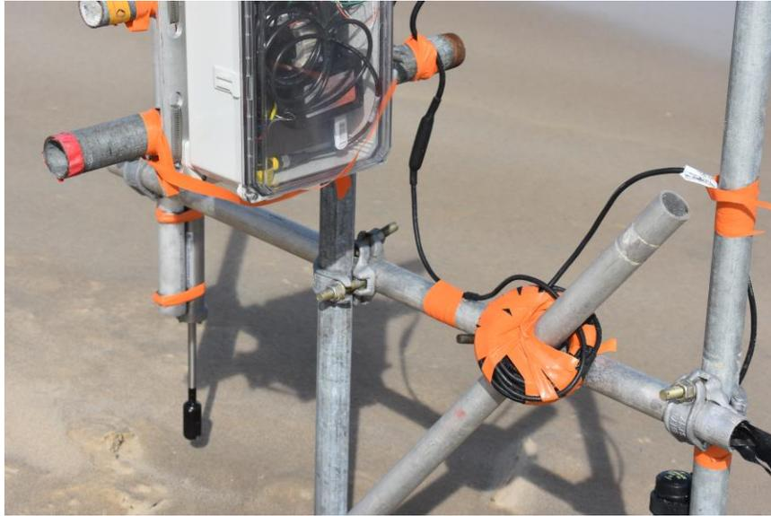
Figure 9 Pipe setup with JFE and ADM
