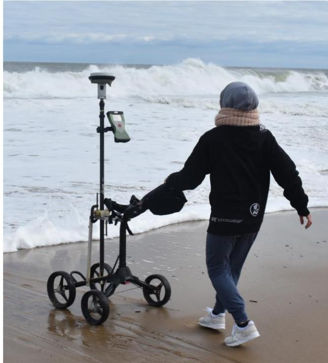
Figure 1 Leica GPS Rover on cart collecting beach profile data
