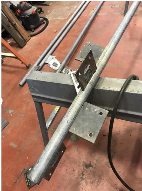
Figure 12 The second fin design for the pipes to resist rotation
