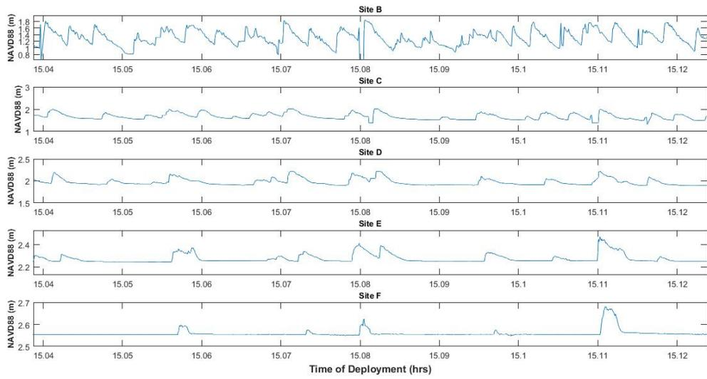
Figure 22 ADM data, relative to the NAVD88, at site B showing the movement of the wave inland, starting at site B until it barely reaches site F.
