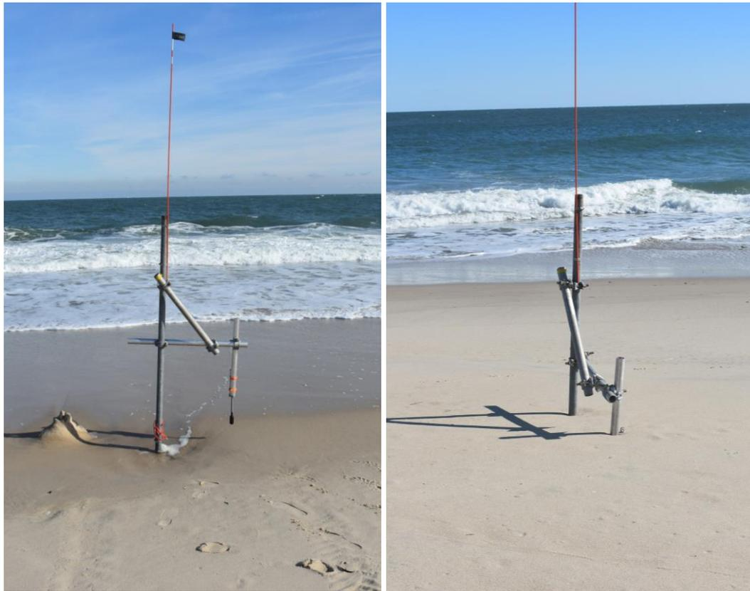
Figure 11 The image on the left shows the original orientation of the pipe, whereas the image on the right is after the pipe rotated 90 degrees clockwise due to the wind.
