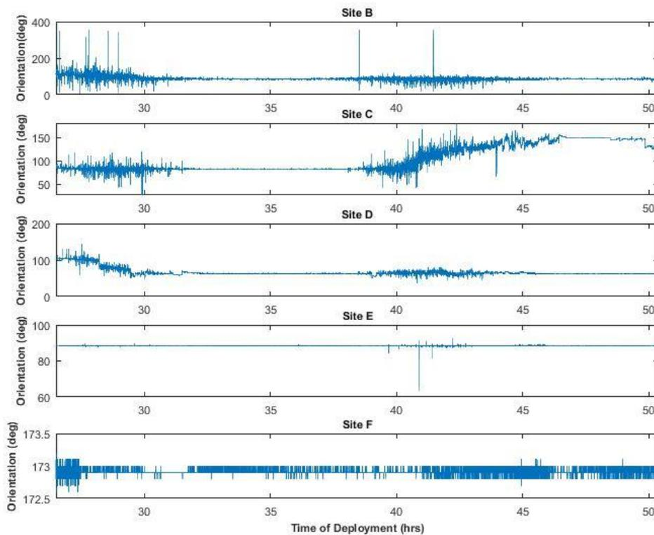
Figure 28 JFE internal compass data throughout the course of the storm, that show how the devices rotated and shifted due to the poles as a result of the storm conditions
