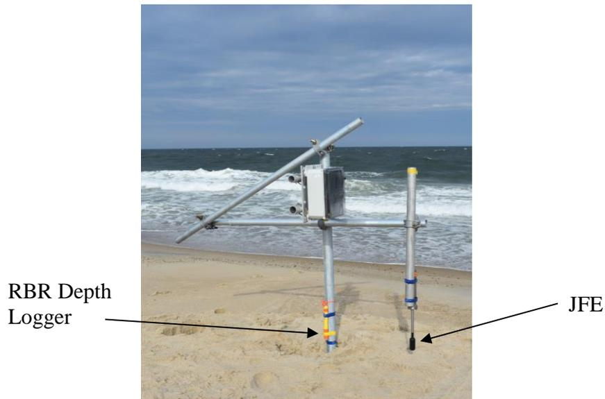
Figure 3 Setup of JFE on pole mount
