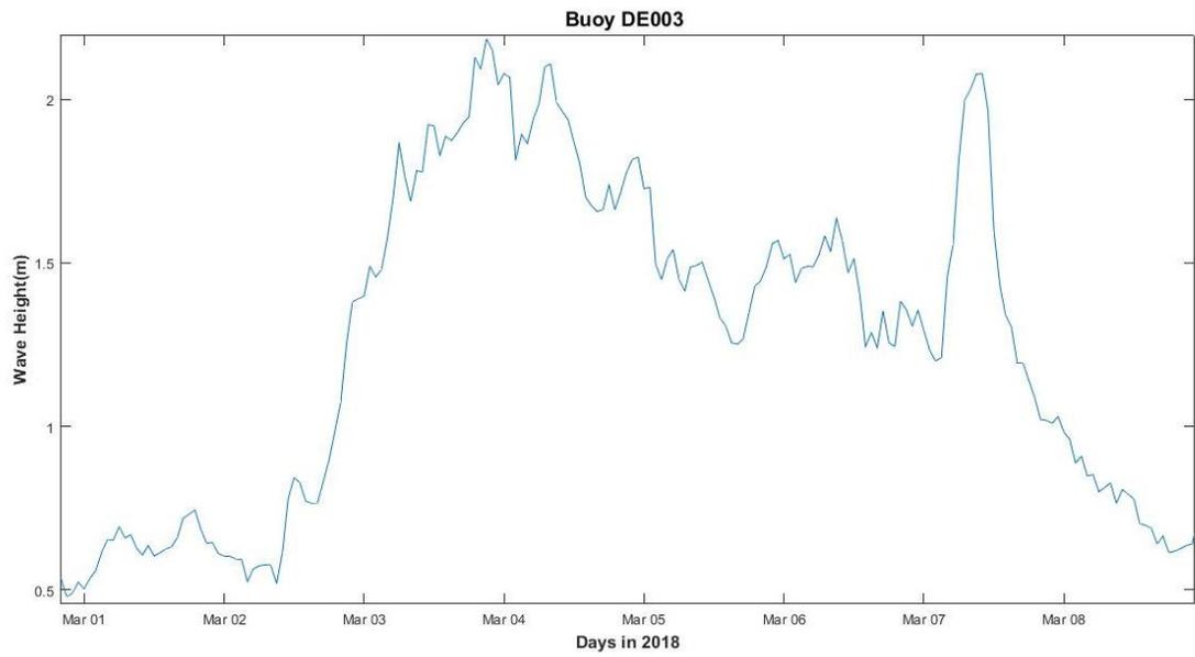
Figure 17 Wave height data collected from buoy DE003 showing the spike in wave heights as Nor' Easter Riley hit the coast of Delaware.
