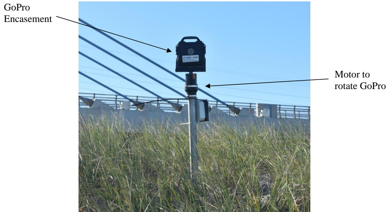
Figure 5 GoPro encasement with motor attachment
