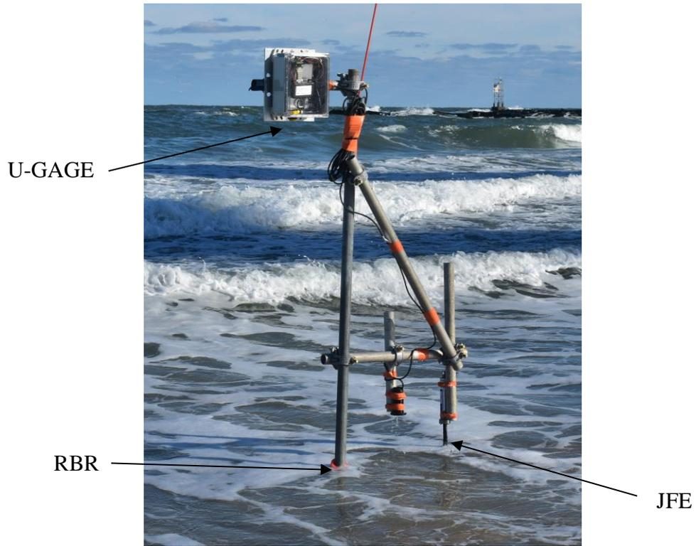
Figure 8 Deployment Pipe Setup with Devices
