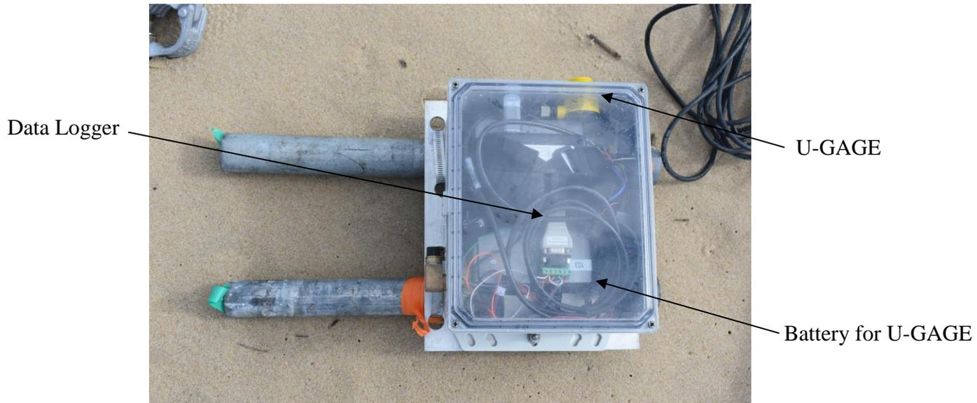
Figure 7 U-GAGE ADM sensor setup within waterproof encasement
