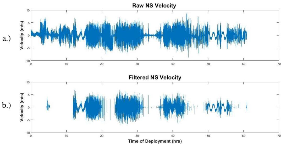
Figure 19 In the top figure (a) it shows the JFE North-South velocity data as it is outputted from the device. Whereas in the bottom figure (b) it shows the same data but with the low frequency pass filter on it as well as removing the data recorded while the JFE was not submerged.
