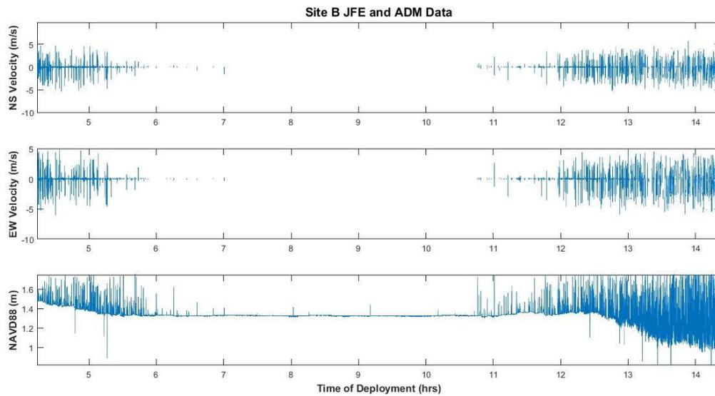
Figure 20 Data collected at site B from the ADM and JFE, showing the clear differentiation of when the tide comes in and the JFE becomes submerged and recording velocities as well as the ADM showing wave activity.
