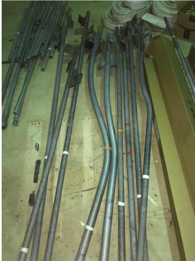
Figure 25 Deformation of the pipes used at each site for Nor' Easter Toby, the pipes with the more drastic curved shape came from sites A through C.
