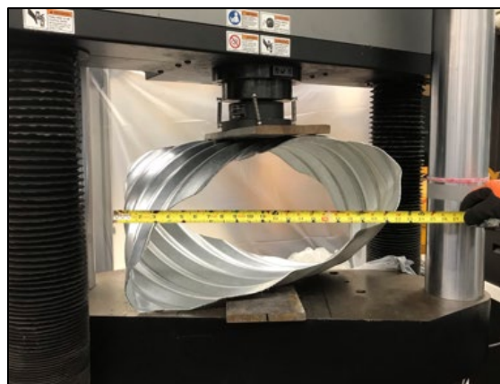
(b) Liner Pipe after Loading.
