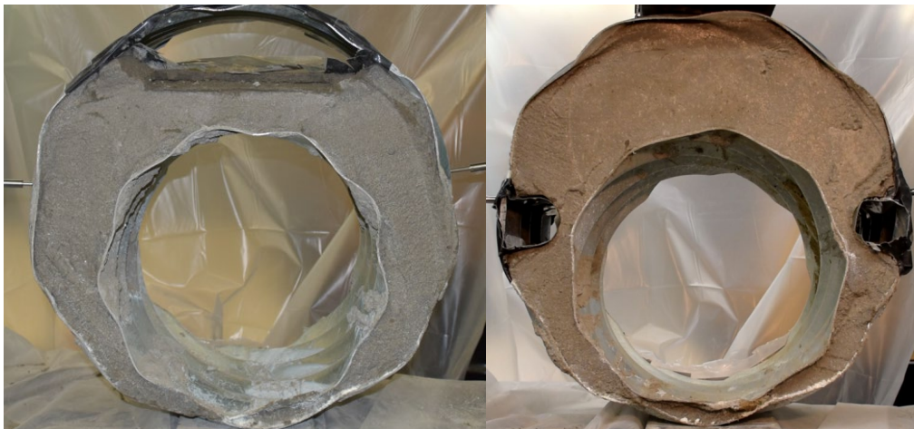
Figure F.24: Sliplined Culvert Specimens: One with a Void at Crown ( left ) and One with Two Voids at the Springline ( right ).
