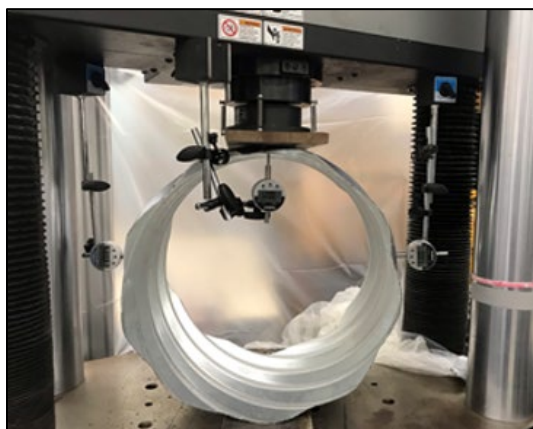
(a) Setup for Liner Pipe Loading.
