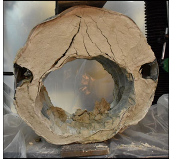
Figure E.59: Sliplined Culvert using C40 Cellular Grout with Voids at the Springline: Before ( left ) and After ( right ) Parallel-plate Load Test.
