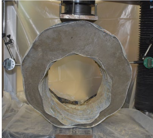
Figure 8: Typical Setup for a Parallel-Plate Loading Test
