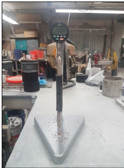
(a) Invar Bar in Length Comparator. (b) Length Comparator with Grout Sample.
