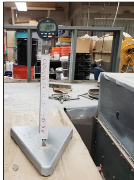
(a) Invar Bar in Length Comparator. (b) Length Comparator with Grout Sample.
