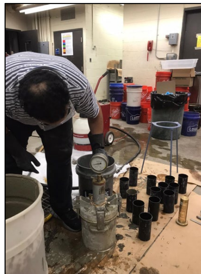
(b) Conducting Air Content Test.
