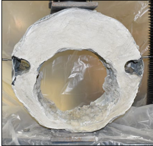
Figure E.59: Sliplined Culvert using C40 Cellular Grout with Voids at the Springline: Before ( left ) and After ( right ) Parallel-plate Load Test.
