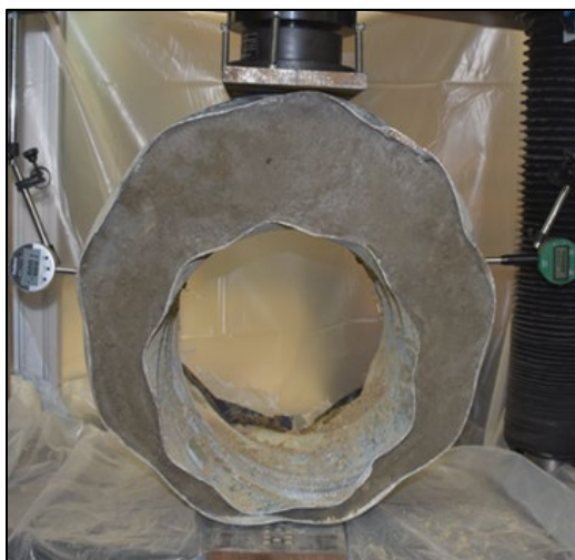
Figure E.54: Sliplined Culvert Using CLSM Grout Mix A, Before ( left ) and After ( right ) Parallel-plate Load Test.
