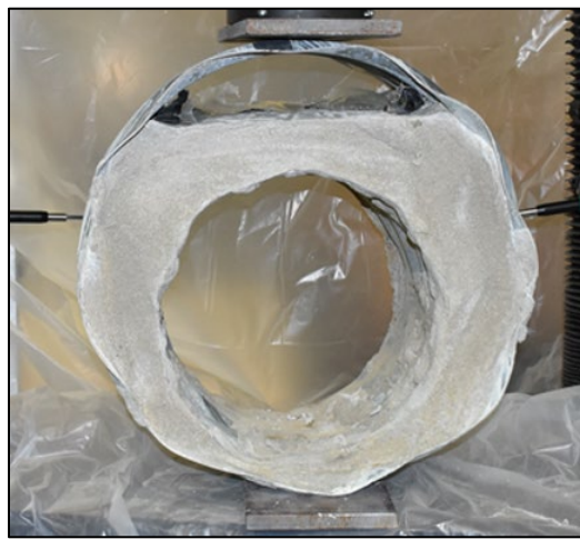
Figure E.60: Sliplined Culvert using C40 Cellular Grout with Voids at the Crown: Before ( left ) and After ( right ) Parallel-plate Load Test.
