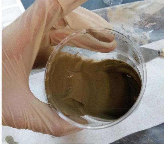
Figure A.14: Two-component grout after gelling (Shah et al. 2018).
