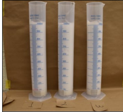
(b) Measuring Foam Density
