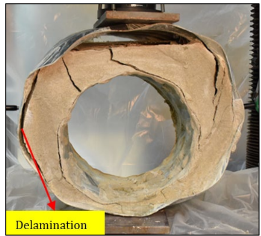
Figure E.60: Sliplined Culvert using C40 Cellular Grout with Voids at the Crown: Before ( left ) and After ( right ) Parallel-plate Load Test.
