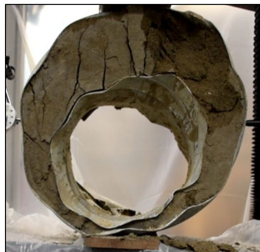
Figure E.54: Sliplined Culvert Using CLSM Grout Mix A, Before ( left ) and After ( right ) Parallel-plate Load Test.
