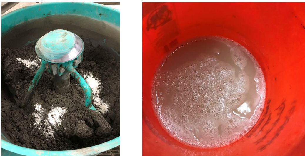
Figure F.3: Mixing Fill Flow: Adding Powder Directly to the Mix (left), Mixing Fill Flow with Water Prior to Adding it to the Mix (right).
