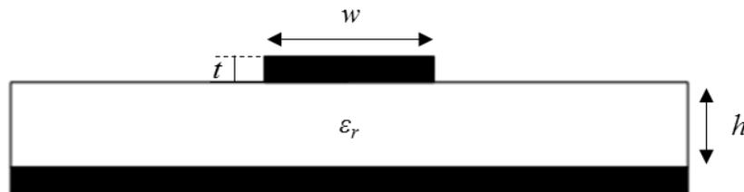
Figure 4.3 Microstrip transmission line.
