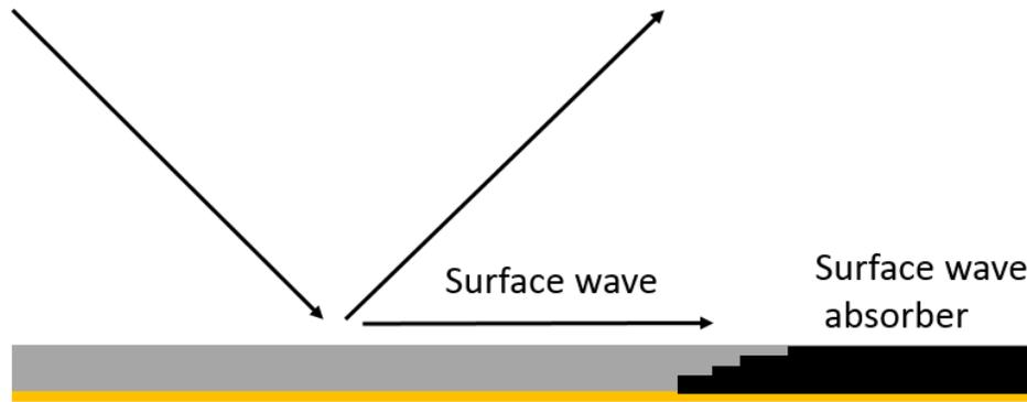
Figure 1.3 Illustration of surface wave absorber.
