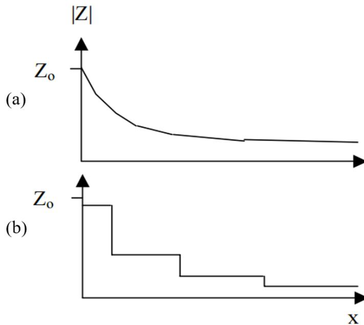
Figure 1.2 Continuous (a) and discrete (b) impedance tapers used to realize broadband absorbers.
