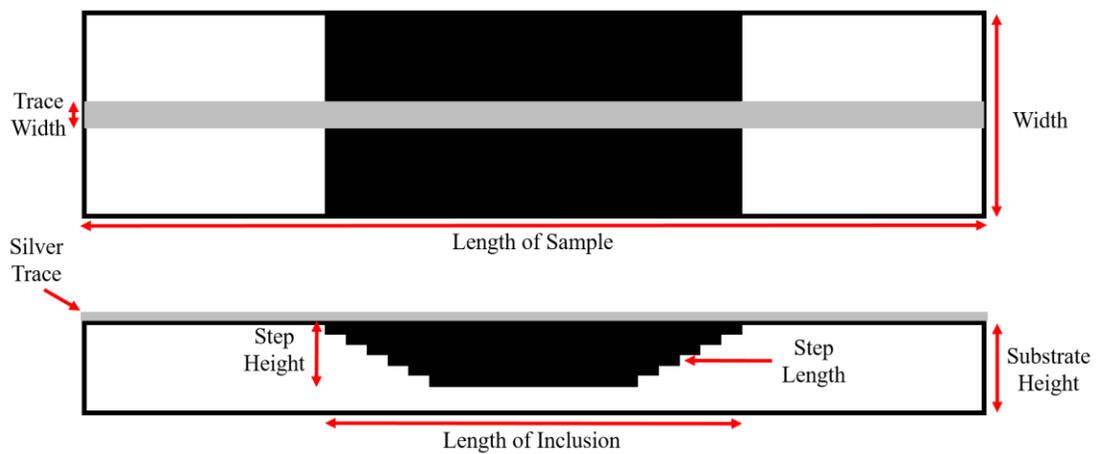
Figure 3.10 Transmission line with DuPont 7082 step slab at top of substrate, top view (top) and side view (bottom).
