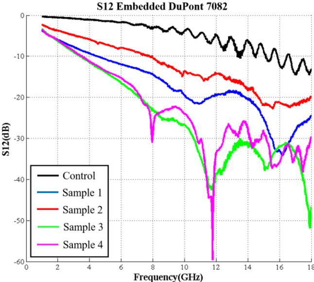
Figure 4.10 S12 plot for nScript printed transmission line samples with DuPont 7082 embedded within the substrate.
