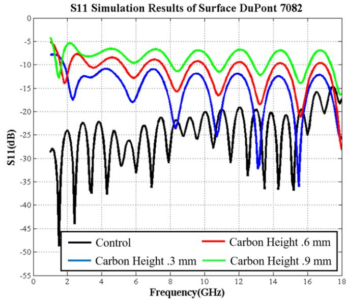
Figure 5.6 S11 plot of simulated transmission line samples with DuPont 7082 slab located at the surface of the substrate. The carbon height is the thickness of the carbon that is located at the surface of a 1.2 mm thick substrate.
