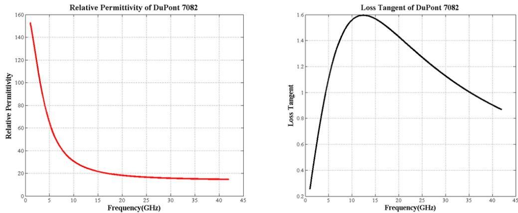
Figure 5.2 Relative permittivity of DuPont 7082 (left) and loss tangent of DuPont 7082 (right).
