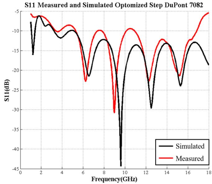
Figure 5.10 Plot of measured and simulated S11 of the optimized step DuPont 7082 in-plane absorber.
