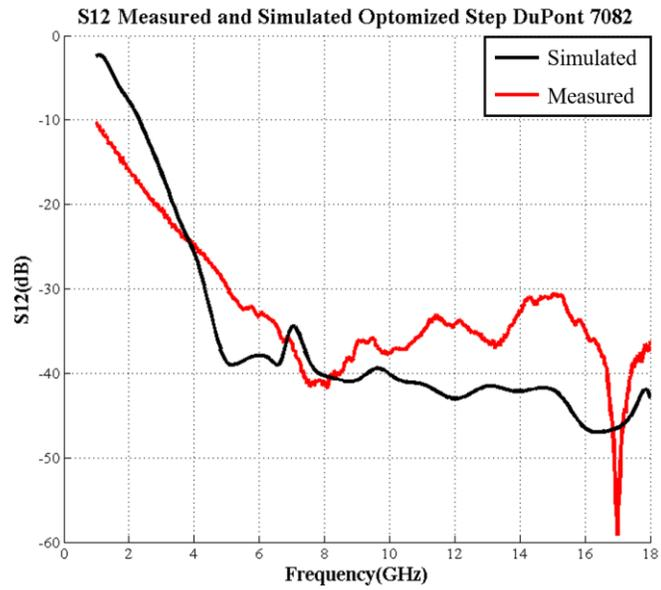
Figure 5.9 Plot of measured and simulated S12 of the optimized step DuPont 7082 in-plane absorber.
