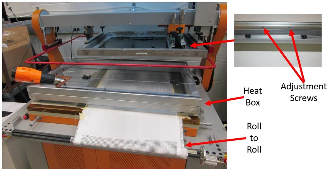
Figure 3.3 Screen printer modifications.
