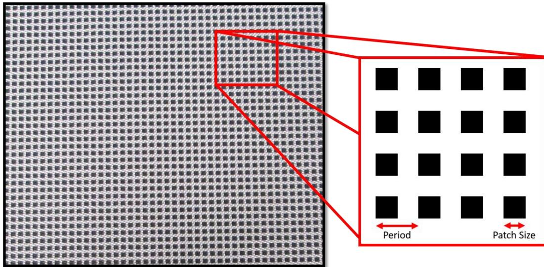
Figure 3.4 Screen printed pattern deposited onto s-glass.
