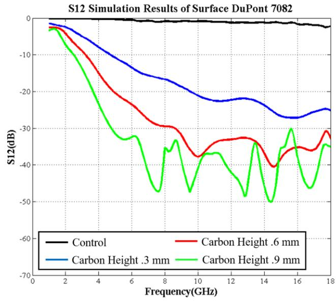
Figure 5.5 S12 plot of simulated transmission line samples with DuPont 7082 slab located at the surface of the substrate. The carbon height is the thickness of the carbon that is located at the surface of a 1.2 mm thick substrate.
