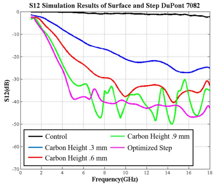
Figure 5.7 S12 plot of simulated transmission line samples with DuPont 7082 slab located at the surface of the substrate and optimized step slab.
