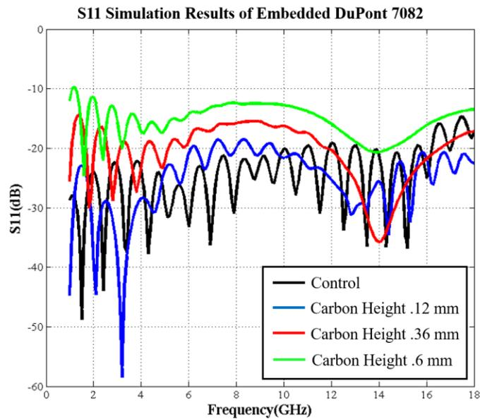
Figure 5.4 S11 plot of simulated transmission line samples with DuPont 7082 slab embedded within the substrate. The carbon height is the thickness of the carbon that is centered within a 1.2 mm thick substrate.
