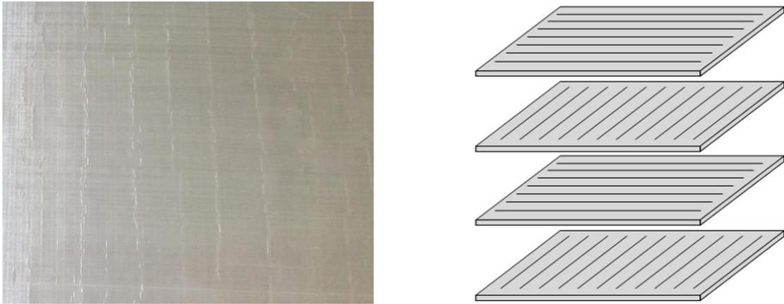
Figure 2.2 Honeywell Spectra Shield 2 SR-3124 (pictured left) and an example of the unidirectional layers that stack to create the substrate (pictured right).
