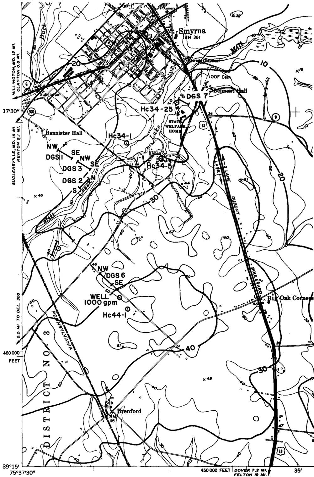
Figure 1. Location of seismic and resistivity stations in Smyrna Area with 10-foot water-table contours (9/1958); after Boggess et al. (1964).
