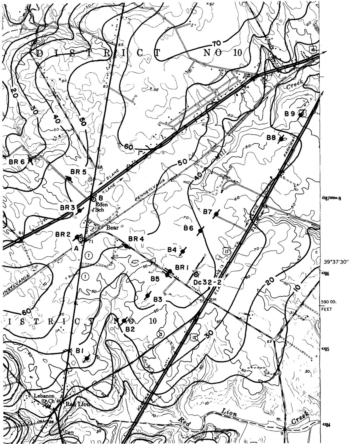
Figure 5. Location of resistivity stations, Bear Area with 10-foot water-table contours (9/1958); after Boggess et al. (1963).
