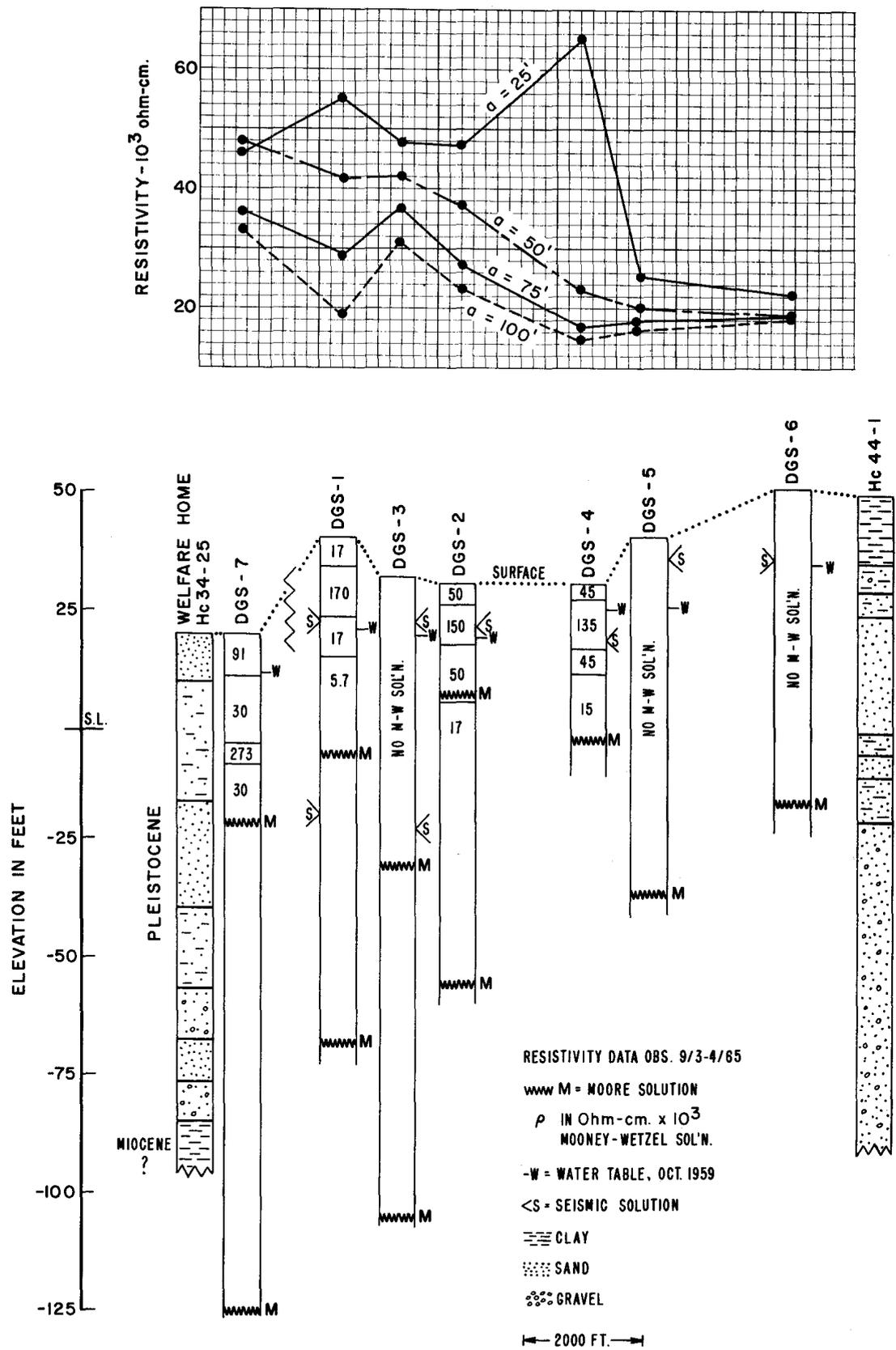
Figure 2. Smyrna Area cross-section.
