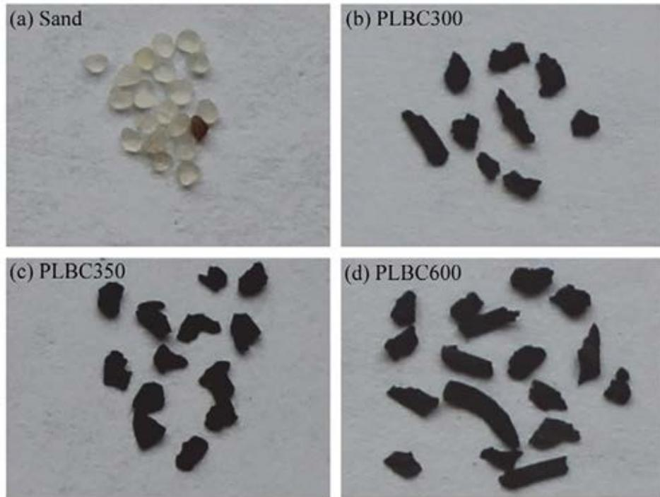
Figure 2-5: Surface geometry of (a) sand, (b) poultry litter biochar (PLBC) pyrolyzed at 300°C (PLBC300), (c) PLBC at 350°C (PLBC350), and (d) PLBC at 600°C (PLBC600). All particles collected between #30 (0.595mm opening) and #35 sieves (0.5-mm opening).
