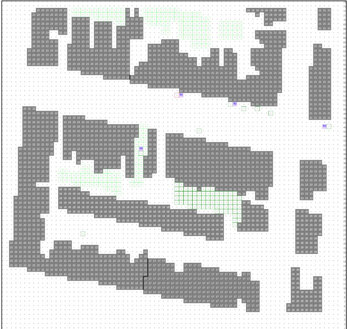
Figure 3.1: Receptor Locations. Receptors are represented as purple cells with abbreviated name (i.e. Garden Sensor = “GS”, Receptor 1 = “R1”, Receptor 2 = “R2” and Receptor 3 = “R3”). The ActualGarden model is shown, but the receptor location is unchanged in each model.
