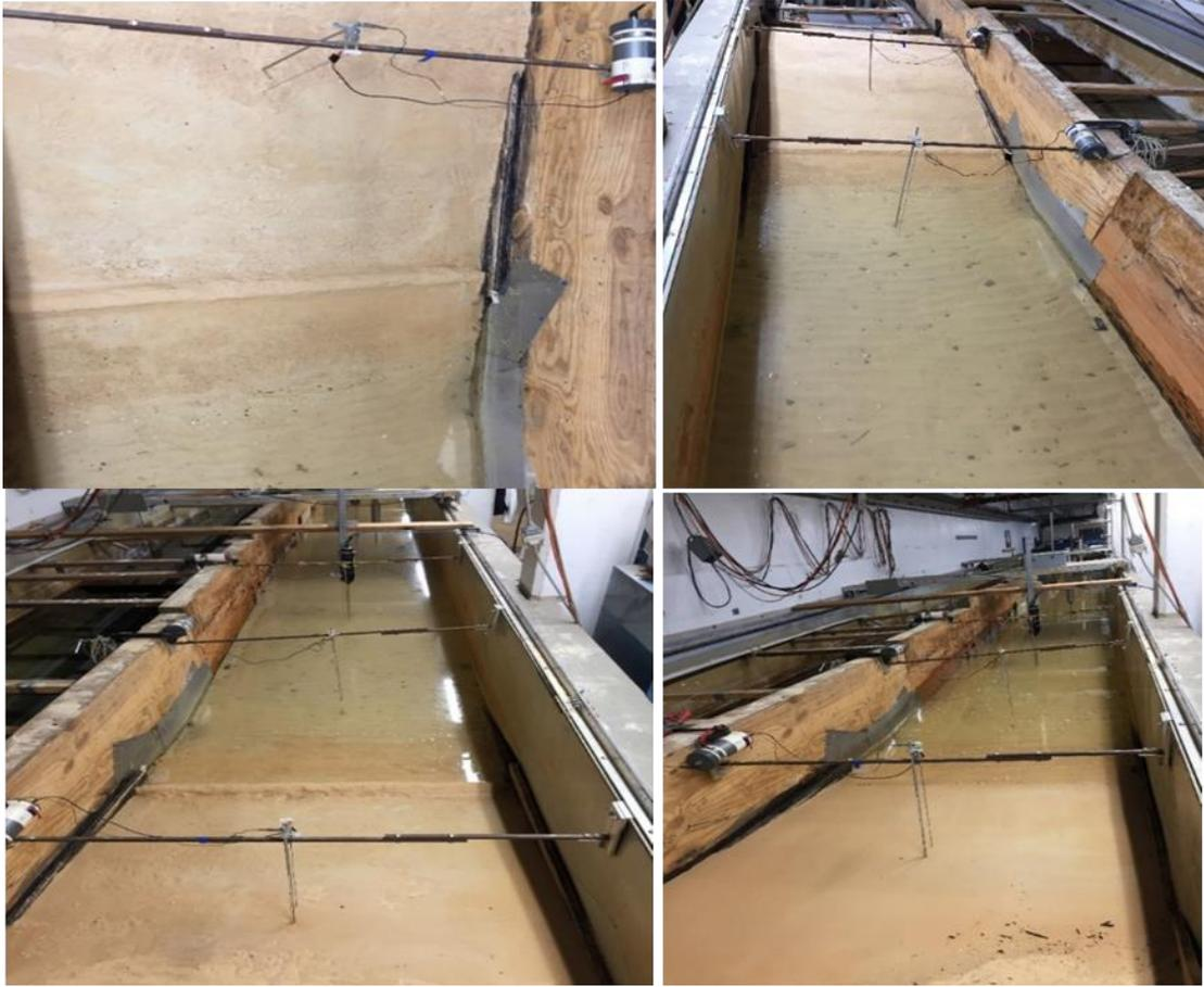
Figure A.12: Placed sand near the shoreline for N test with no wave overtopping and overwash
