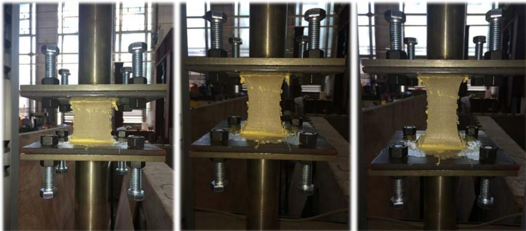
Figure 3.6 Foam Specimen Extension During Tension Testing
