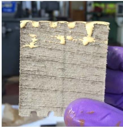
Figure 3.3 Section View of Foam Grooves; Epoxy Coated (top) and Vacant (bottom)
