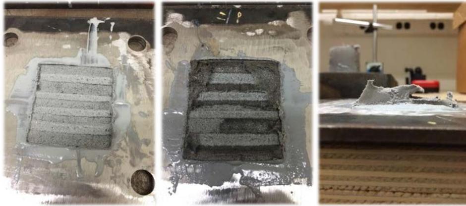
Figure 3.8 Bond Failure (left); Foam Groove Failure (center); Foam Body Failure (right)
