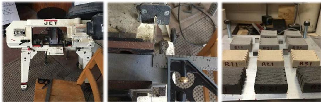
Figure 2.1 Band Saw and Foam Roll (left and center); Specimen Labelling System (right)
