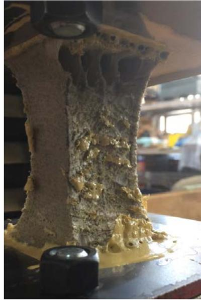
Figure 3.9 Specimen Experiencing Groove Failure
