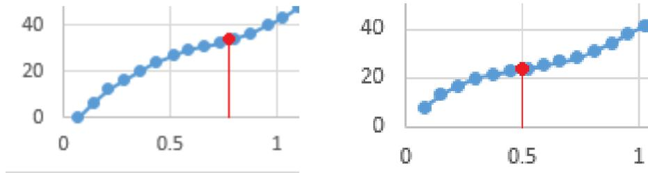
Figure 3.12 Force-Deflection Inflection Points, 0.8” for Room (left); 0.5” for Elevated (right)
