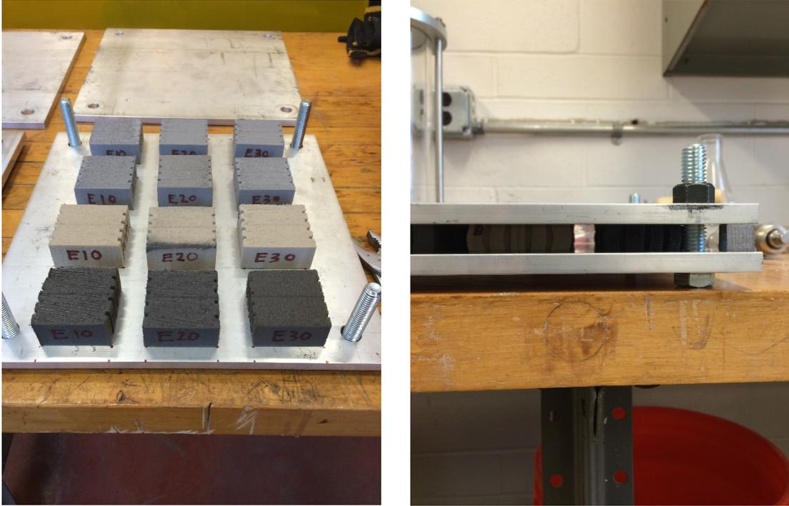
Figure 2.4 Specimens Loaded in Open Apparatus (Left); Specimens Compressed to 0.5 Inches (Right)
