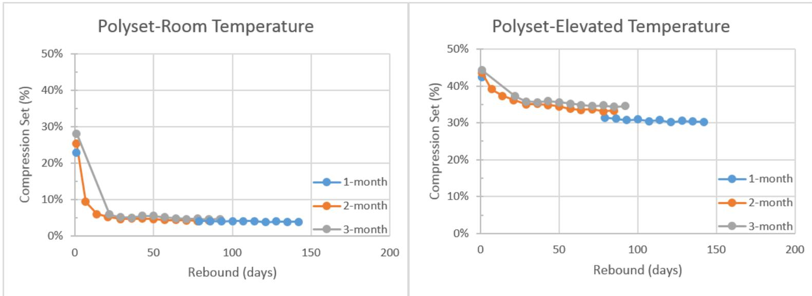
Figure 2.7 Compression Set Data for Extended Rebound Durations
