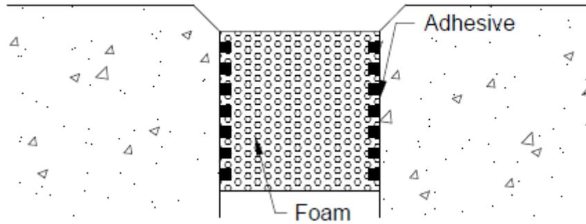
Figure 1.3 Typical CCF Cross Section
