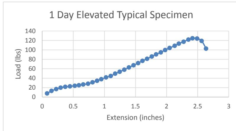
Figure 3.11 Typical Force-Deflection Plots for 1 Day Room and Elevated Specimens
