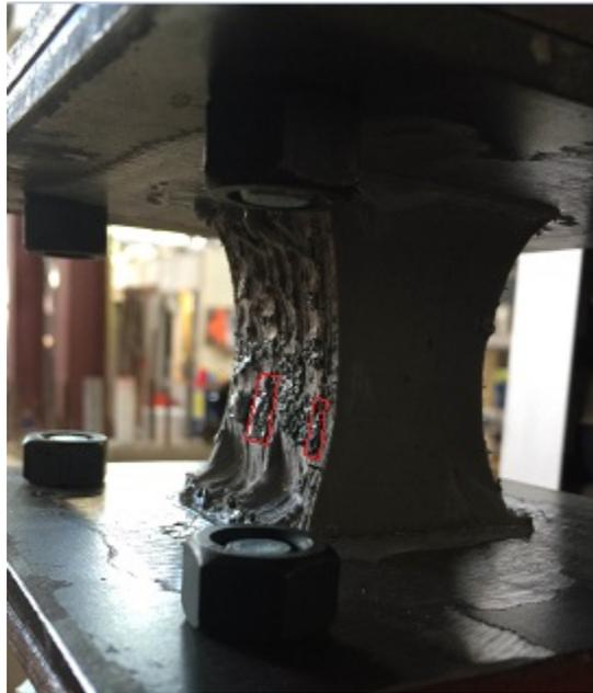
Figure 3.10 Foam Body Failure; Tear Propagation due to Dried Excess Epoxy
