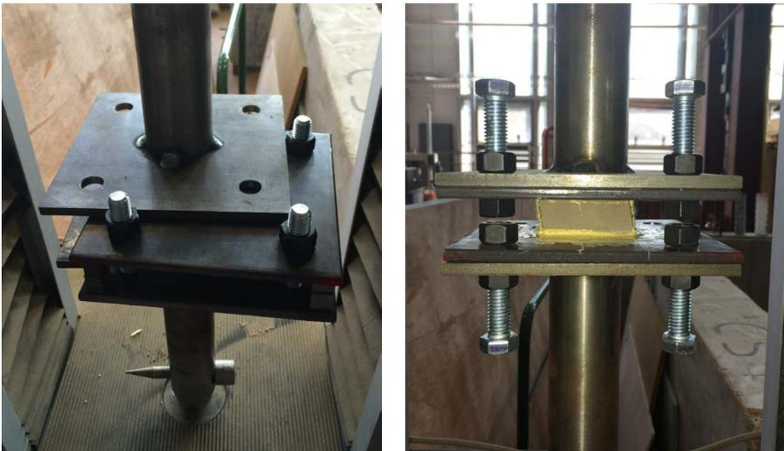
Figure 3.5 Preventing Rebound While Loading Specimen (left); Loaded Specimen (right)
