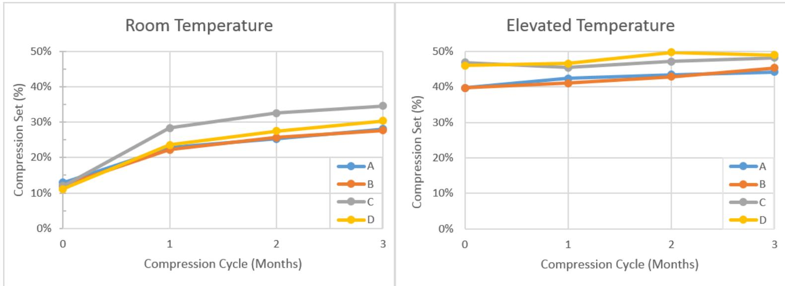
Figure 2.6 Compression Set for Room Temperature Trials (Left); Compression Set for Elevated Temperature Trials (Right)
