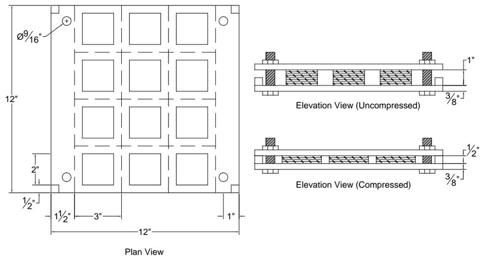
Figure 2.2 Design Sketch of Testing Apparatus
