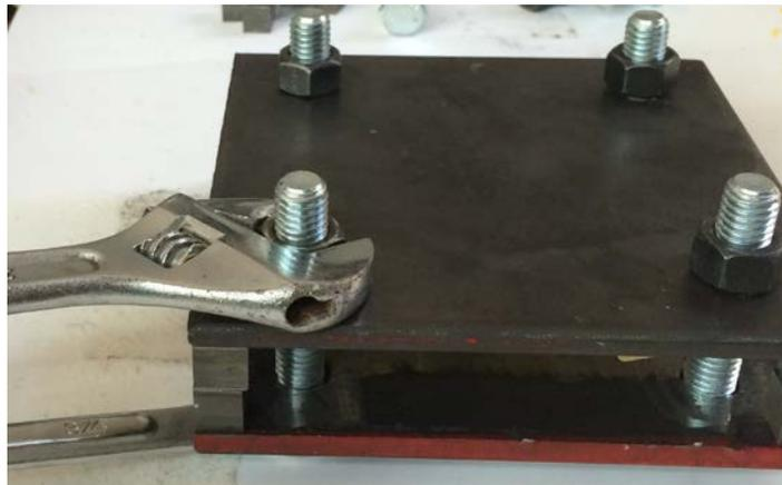
Figure 3.1 Single Compression/Tension Specimen Fixture in Closed Position
