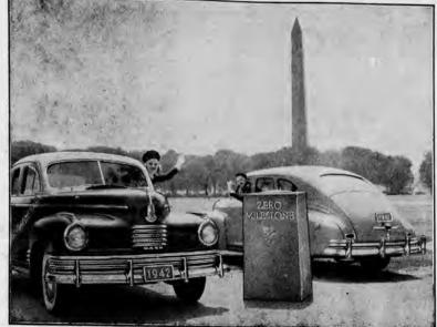
Here are two of the three series of cars being introduced by Nash for 1942. Fore, is the Nash Ambassador Six, a big car driven by a valve-in-head, six-cylinder power plant which incorporates something new in auto engines—a
