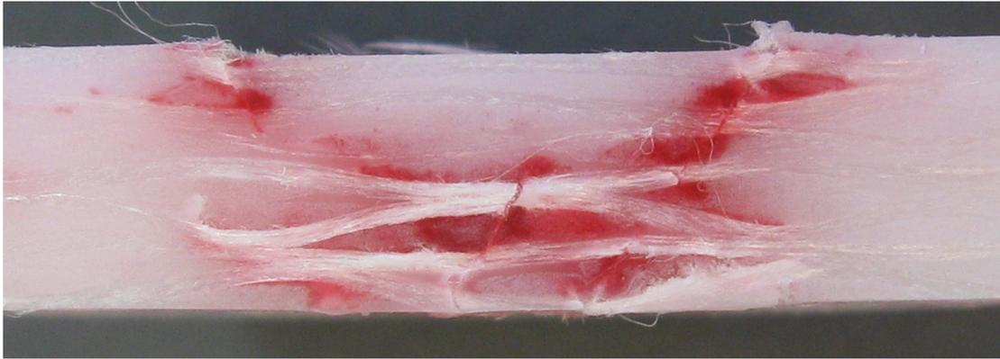
**Figure 2.6 – Typical sectioned specimen (11.09-mm punch, 5.08-mm sample)**
