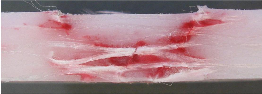
**Figure 3.1 – Confined compression failure (11.09-mm punch, 5.08-mm sample)**
