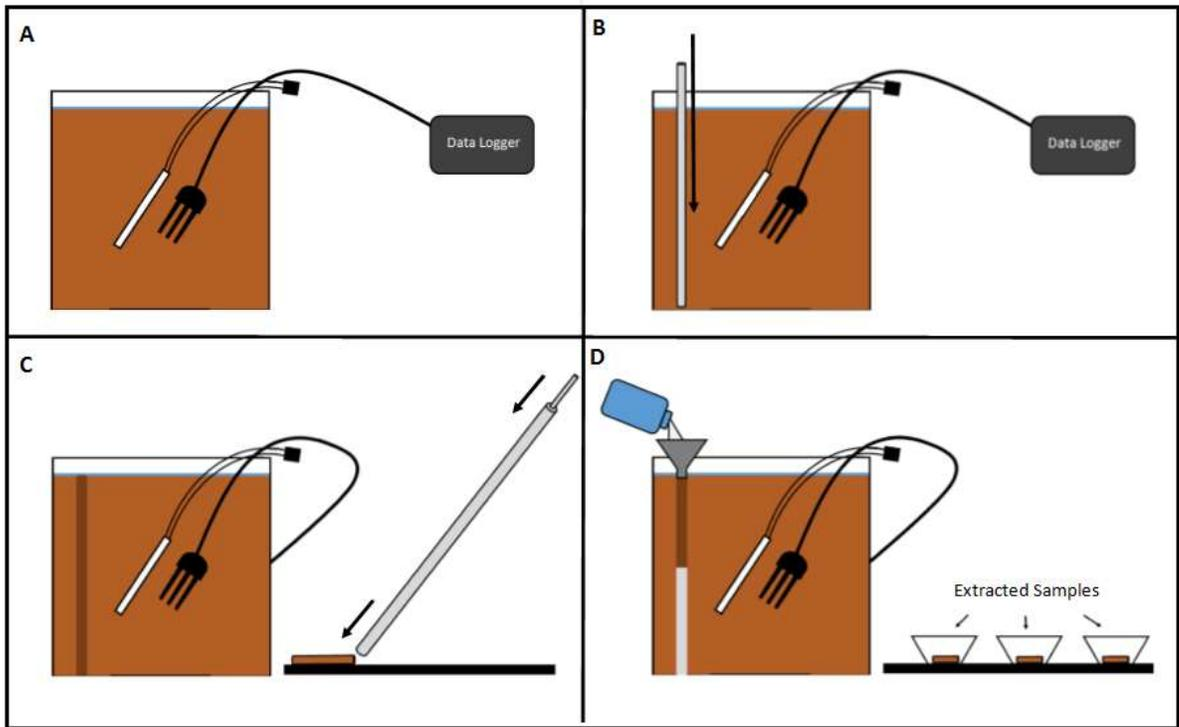
Figure 3.11: Schematic of the incubation column sediment extraction in cross section using an aluminum corer. A) Pre-collection incubation column cross section. B) Sediment extraction corer was used to core out a 1/4" core for the entire column height. C) Sample core was deposited and divided into "Top", "Bottom", and "Middle" sections. D) Heat-treated bentonite was used to fill the core hole and subsamples were processed.
