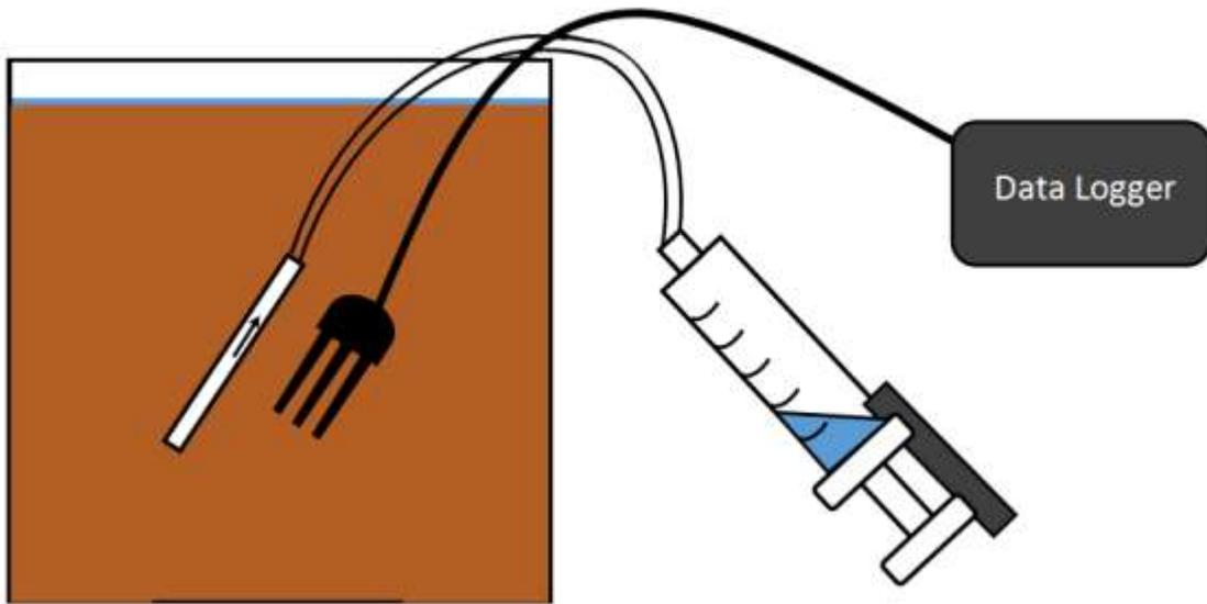
Figure 3.10: Schematic of the incubation column pore water extraction in cross section. Once a vacuum was applied to micro-rhizon sampler (white rectangle) by the extending and locking the extraction syringe, porewater flowed through the sampler and was collected in the syringe. After sufficient water volume was collected, the sample was decanted to storage containers. The moisture probe (black three-pronged probe) remained intact throughout collection process.
