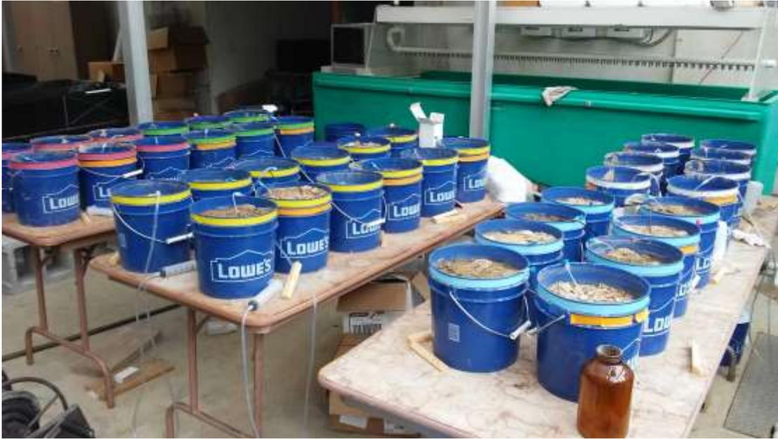
Figure 3.8: Incubation columns set up at the greenhouse of the Stroud Water Research Center, Avondale, PA. Incubation columns were grouped by sediment type (indicated by top layer of colored tape on each bucket), but Regime treatment columns were in an alternating order (e.g., Column order of Regime 1 (no bottom tape label), Regime 2 (orange tape label), Regime 1, Regime 2, etc.).
