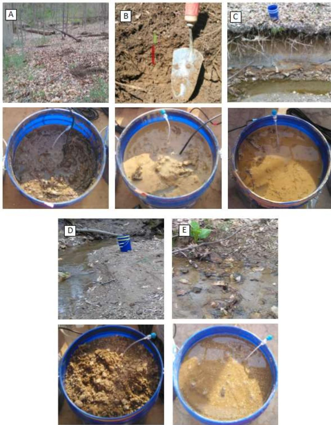
Figure 3.2: POM source sites and corresponding incubation columns. The POM sources types are as follows: A) Forest Floor Humus; B) Upland Mineral A Horizon; C) Stream Bank (composite of exposed A and B horizons); D) Storm Deposit; and E) Stream Bed.
