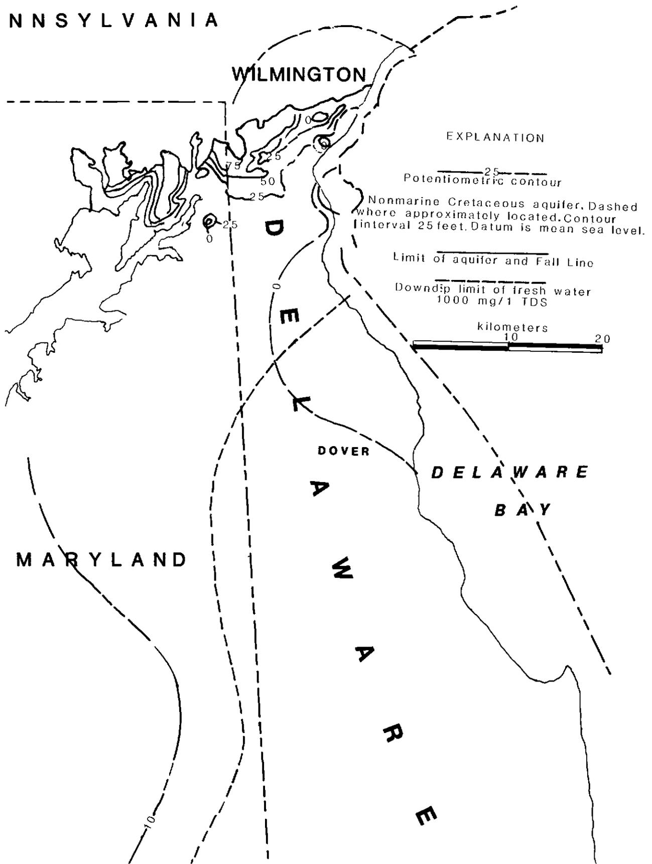
Figure 8. Potentiometric surface of the Potomac Formation from Cushing et al. (1973).
