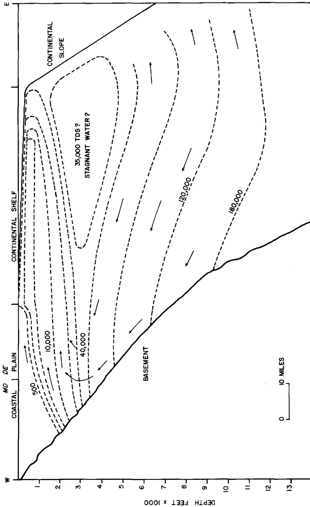
Figure 6. Schematic presentation of salinity distribution and ground-water flow.
