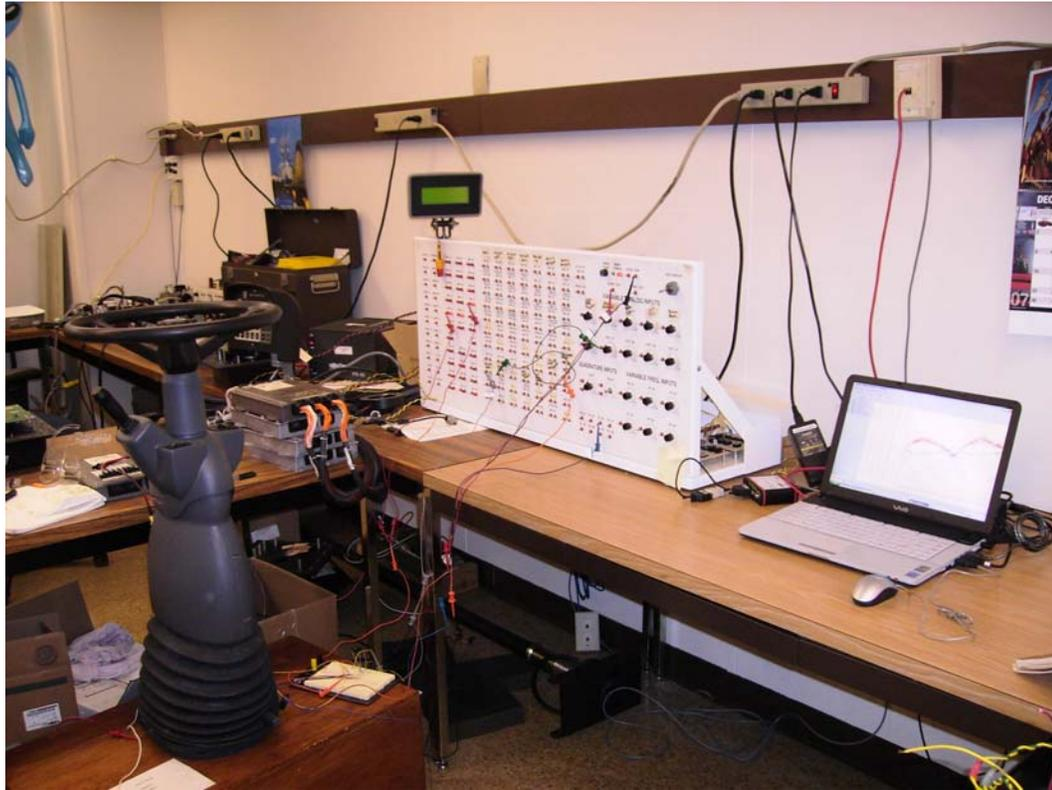
**Figure 3.5:** A picture of the testbed for data acquisition of steering column system identification experiment.
