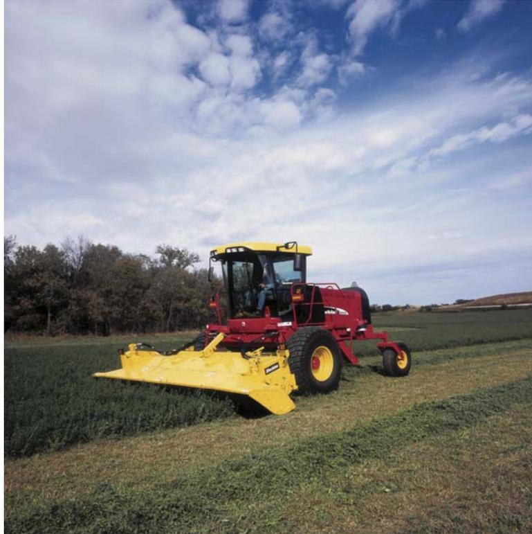
**Figure 2.1:** A New Holland HW365 self-propelled windrower with a 2358 header cutting forage. The rows of crop the vehicle creates are called ‘windrows’, hence the name windrower. Image courtesy of CNH America LLC.
