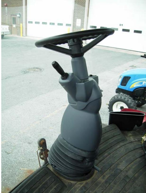
**Figure 2.7:** A modified steering column has been mounted to the cab of the prototype windrower.
