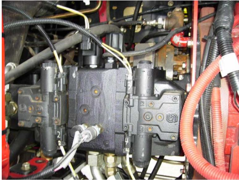
**Figure 2.2:** Picture of an axial piston pump which powers the hydrostatic loop of a self-propelled windrower.
