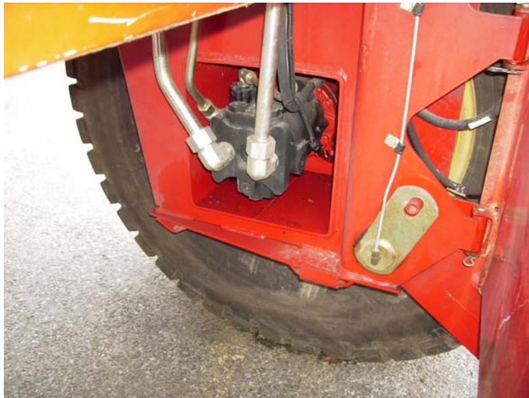
**Figure 2.3:** Picture of an axial piston motor which is powered by an axial piston pump and drives self-propelled vehicle.
