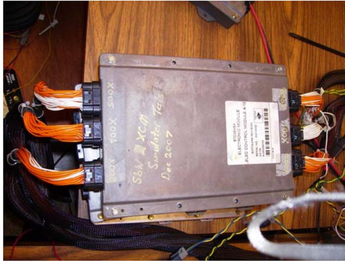
**Figure 2.4:** Picture of vehicle main control module which is onboard the New Holland H series and CaseIH WDX series self-propelled windrowers.
