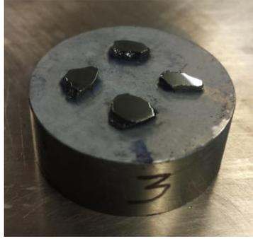
Figure 3-4: Photo of polished crystals mounted on polishing chuck after 0.03  $\mu\text{m}$  alumina polish
