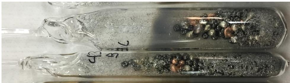
Figure 2-25: Photos comparing ampoule size for 10 and 15 mm ampoules both with 10g of loaded elements.
