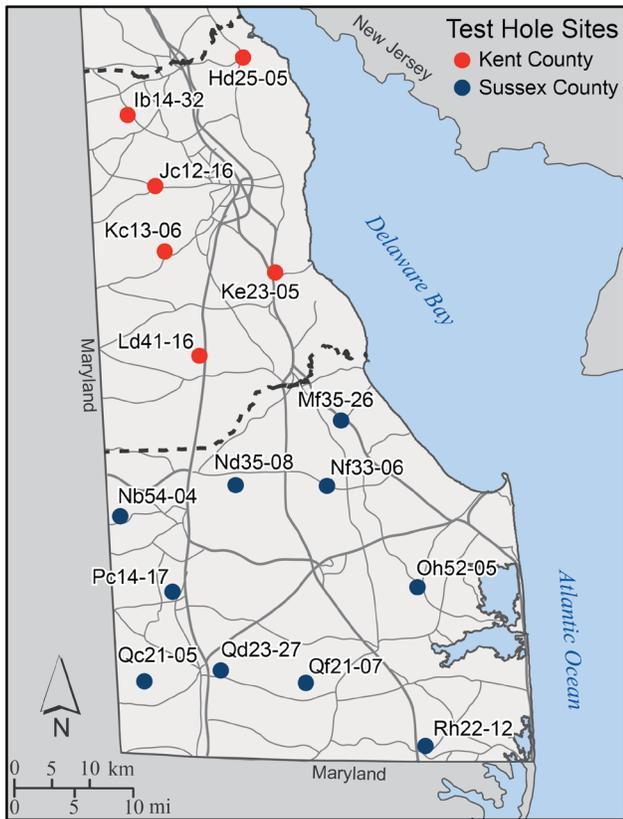
**Figure 6.** Map showing locations of test holes drilled in Kent County for McLaughlin and Velez (2006) and in Sussex County for this study to collect additional geological data on confined aquifer intervals. Site names and depths of test holes for Sussex County are shown on Table 2.
