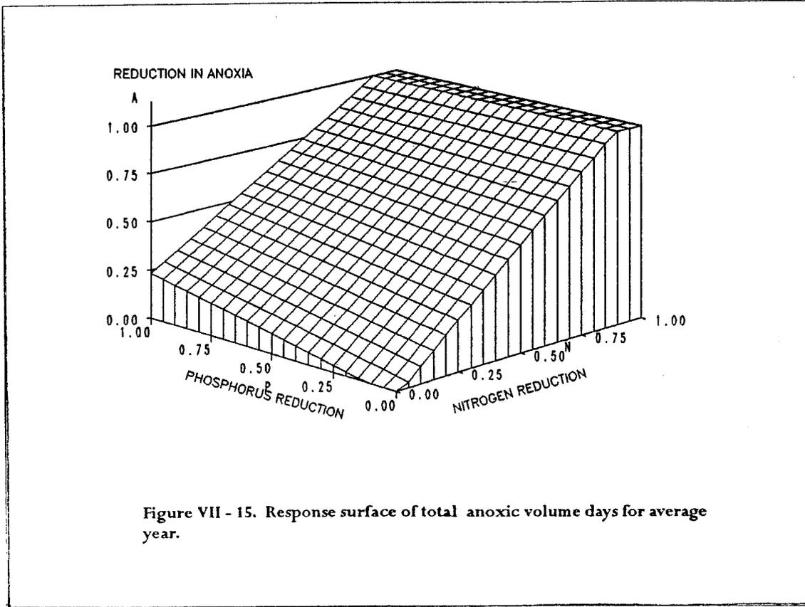
Figure VII - 15. Response surface of total anoxic volume days for average year.
