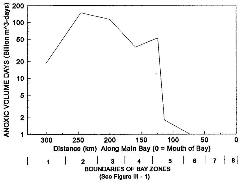
Figure VII - 11. Longitudinal variation of anoxic volume days for Base case total over zone for average year.
