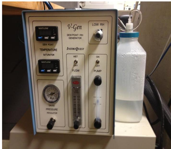
Figure 3-2 V-gen Humidity Generator
