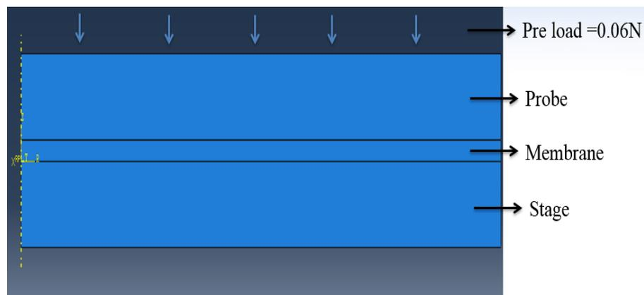
Figure 3-6 Schematic of numerical model for out-of-plane swelling coefficients investigation
