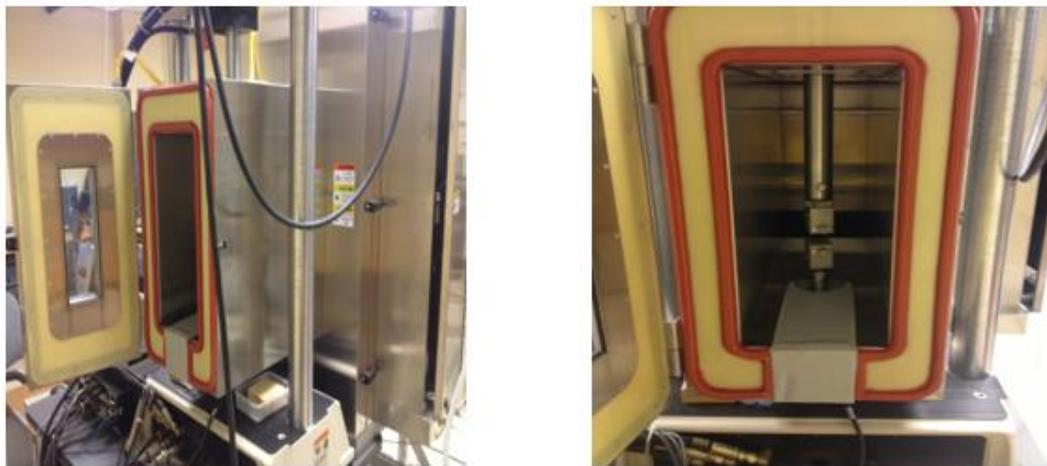
Figure 2-3 MTS testing system with custom designed environmental chamber
