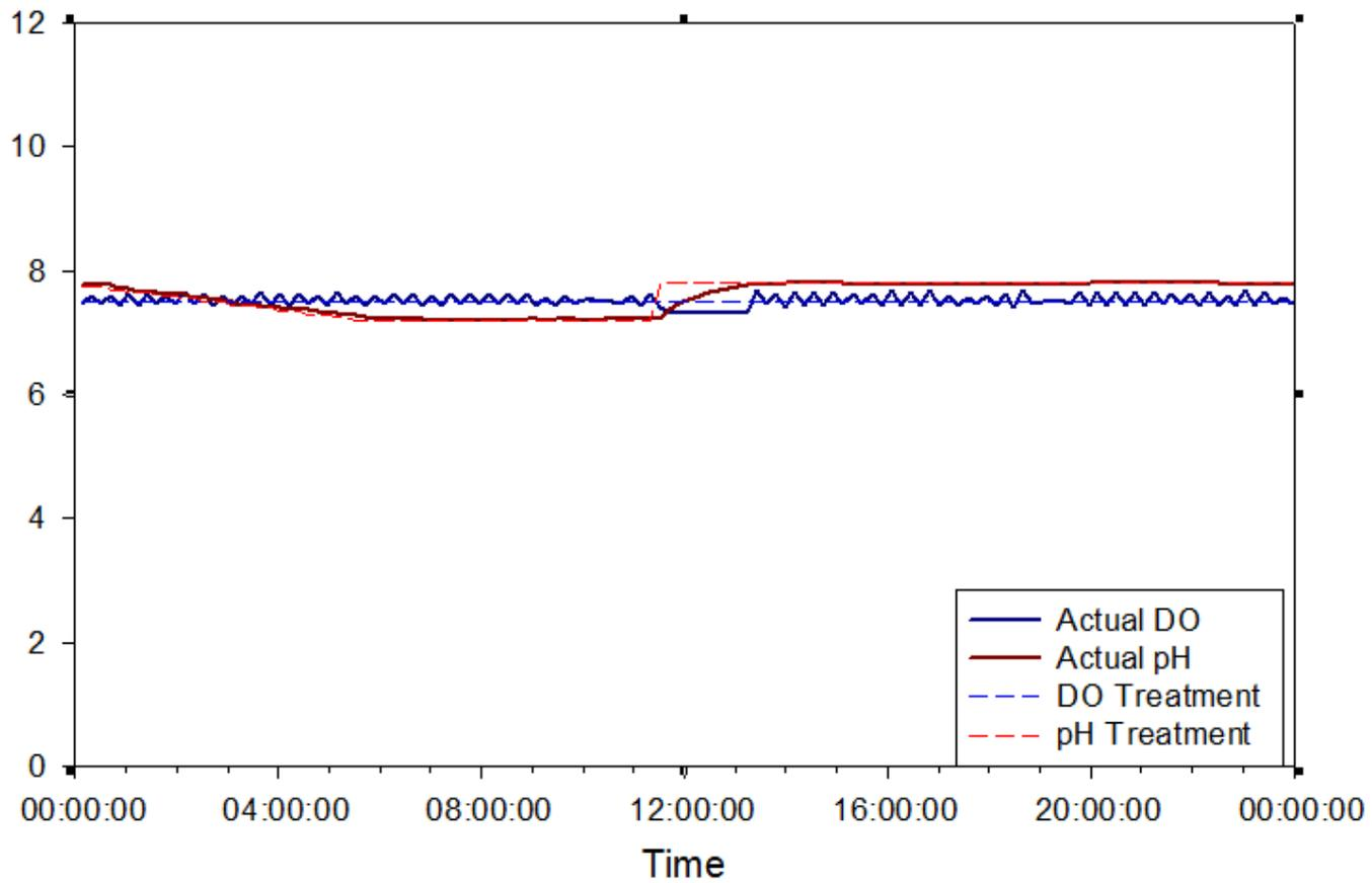
Figure B8: Treatment 8 (Control-DO/N-pH); actual recorded and targeted values over 24 hrs.
