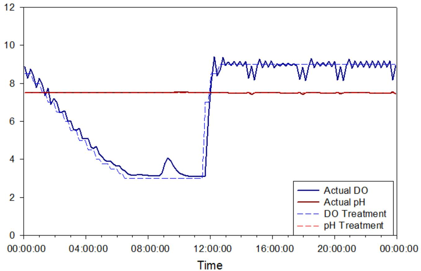
Figure B6: Treatment 6 (N-DO/Control-pH); actual recorded and targeted values over 24 hrs.
